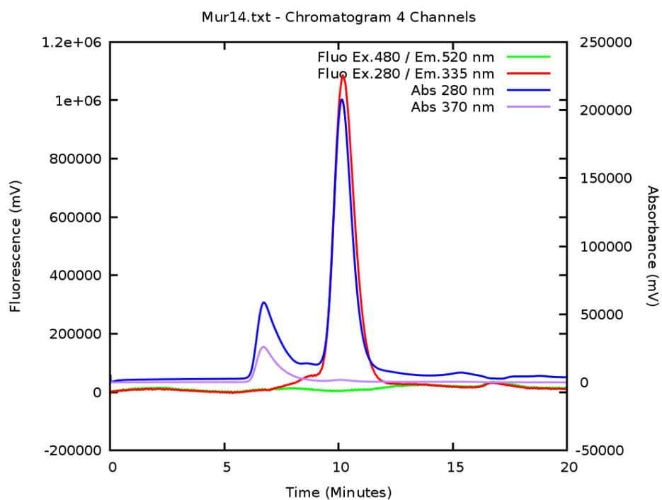
**S7 Fig. Absorbance and fluorescence chromatographic profile on Superdex 75 5/150 GL column of *BcGR* incubated with compound (2).**
