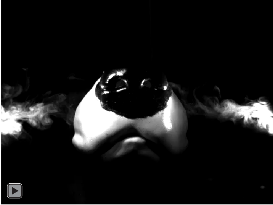
Figure S4. High-speed videography of the dog's nose exhaling theatrical fog (anterior view) shows similar turbulent air jets originating from the nostrils during expiration. This video was filmed at 3000 frames per second.
