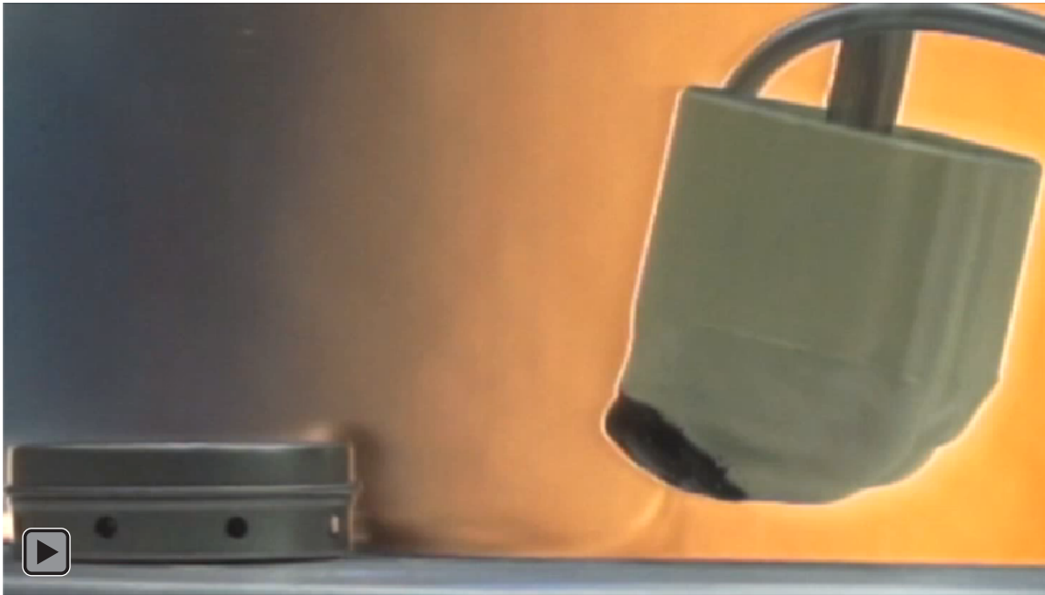
13 Figure S1. Schlieren footage of the biomimetic dog's nose sniffing an acetone-soaked foam plug 14 within a training aid can. The frequency of sniffing is 5 Hz and the sinusoidal flow profile is similar 15 to that of a female Labrador retriever. Click on the video to begin playing.
