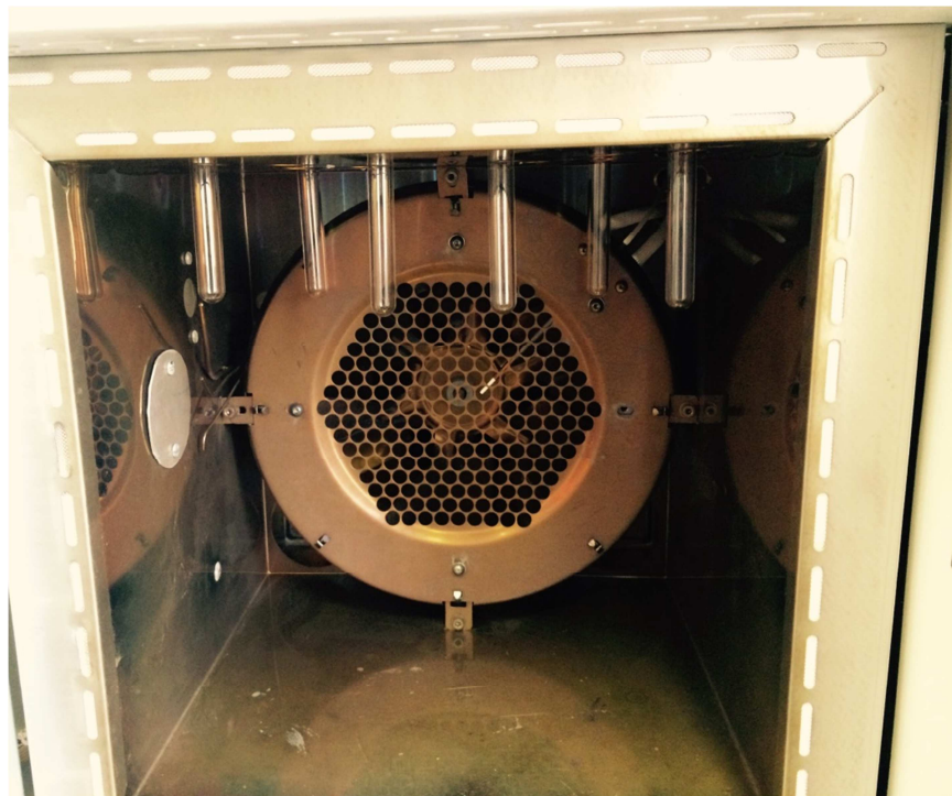
Figure S4. Internal view of the GC oven. Note the 6 disposable 12-mm Pyrex tubes for gypsum sample loading.
