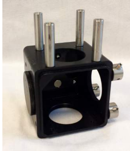
Figure 29: Dichroic filter cube with pockets and 1" posts installed (steps 1-4)
