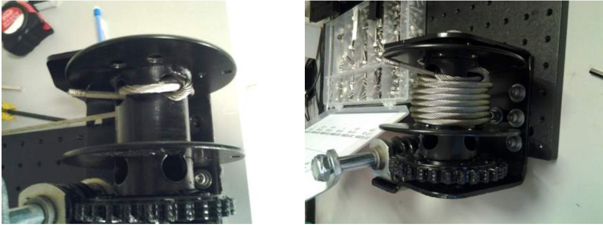
Figure 41: Knot to begin winding steel cable on winch and the wound up steel cable, and overall pulley system
