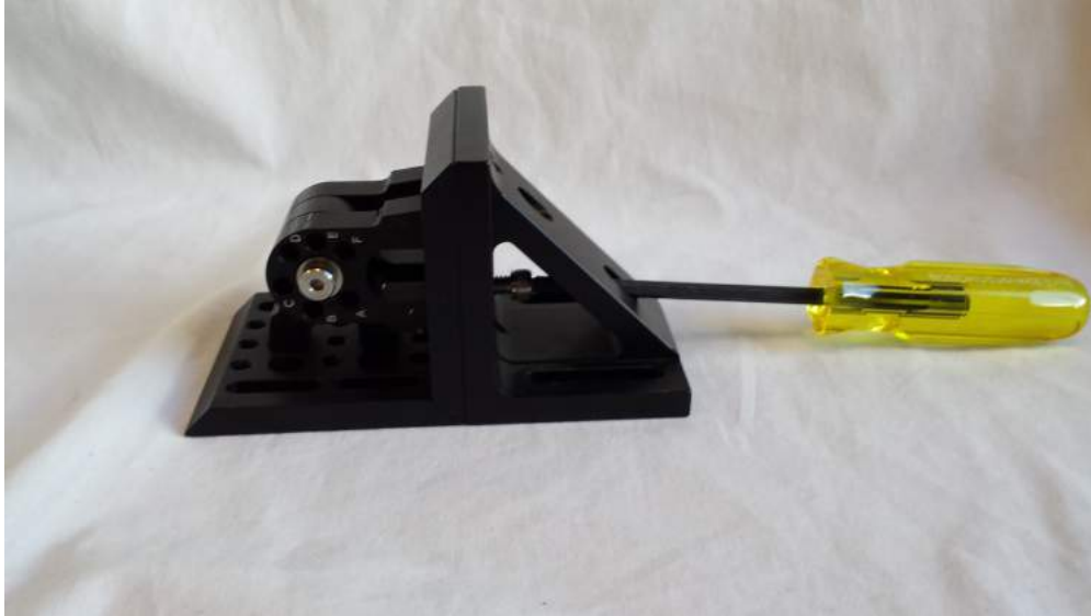
Figure 19: Step 3. screws threaded through the triangular leg of 90 degree bracket
