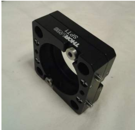
Figure 24: Step 4, with setscrews threaded onto the back plate
