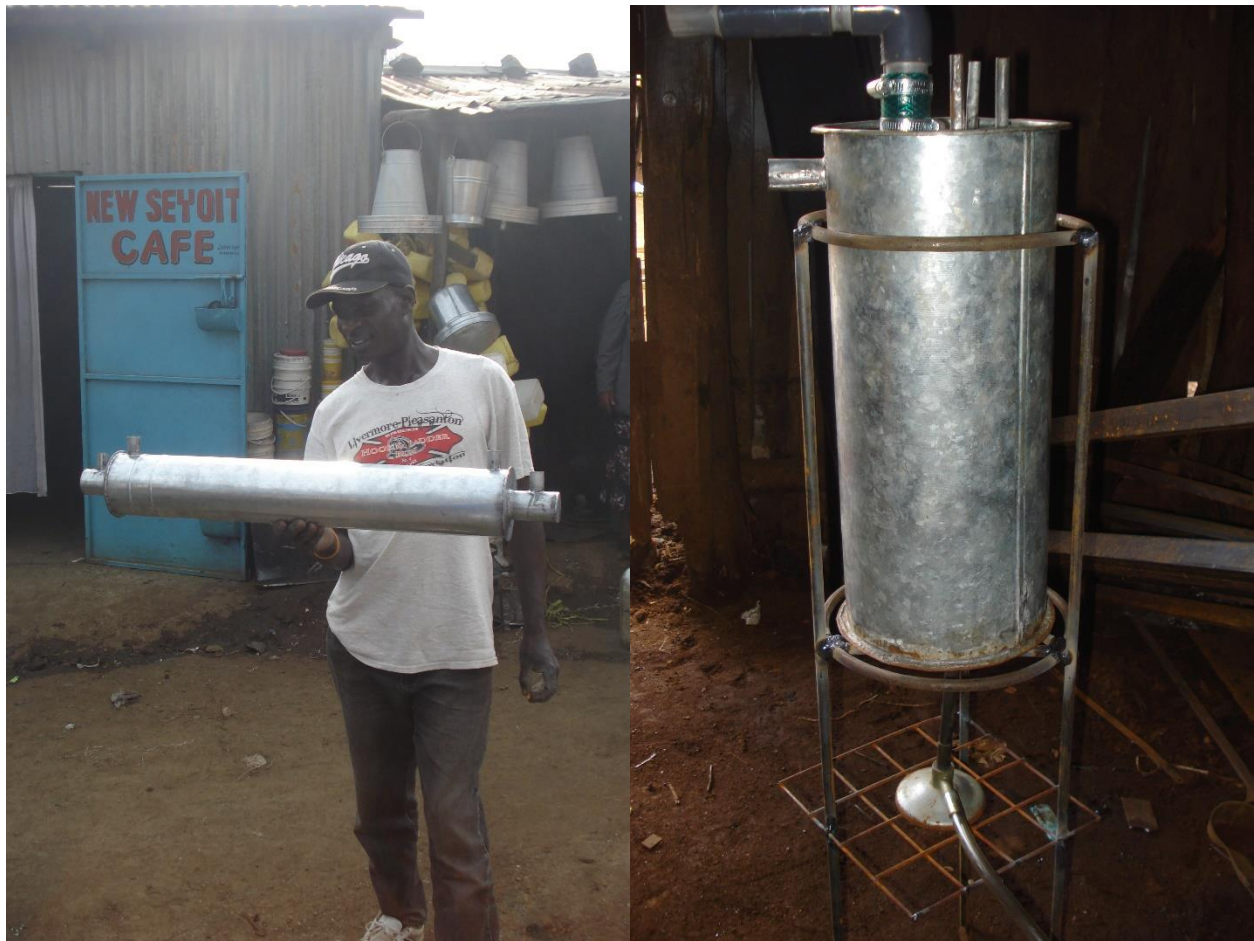
Figure S3. Schematic of heating system (top) and locally fabricated heat exchanger (bottom, left) and heater (bottom, right).
