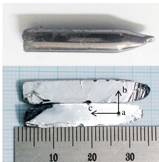
< Figure r5. The photos of Bi doped SnSe single crystal and cleaved sample.>
