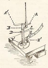
The chin-rest A is attached to a metal tube, BB<sup>1</sup>, on which it rotates horizontally (A<sup>1</sup>) so as to be utilized for the examination of either eye. The tube BB<sup>1</sup> telescopes into the hollow metal pedestal C, and has a vertical range of movement of 4 inches, within which it can be fixed at any point by a screw D with a milled head.
