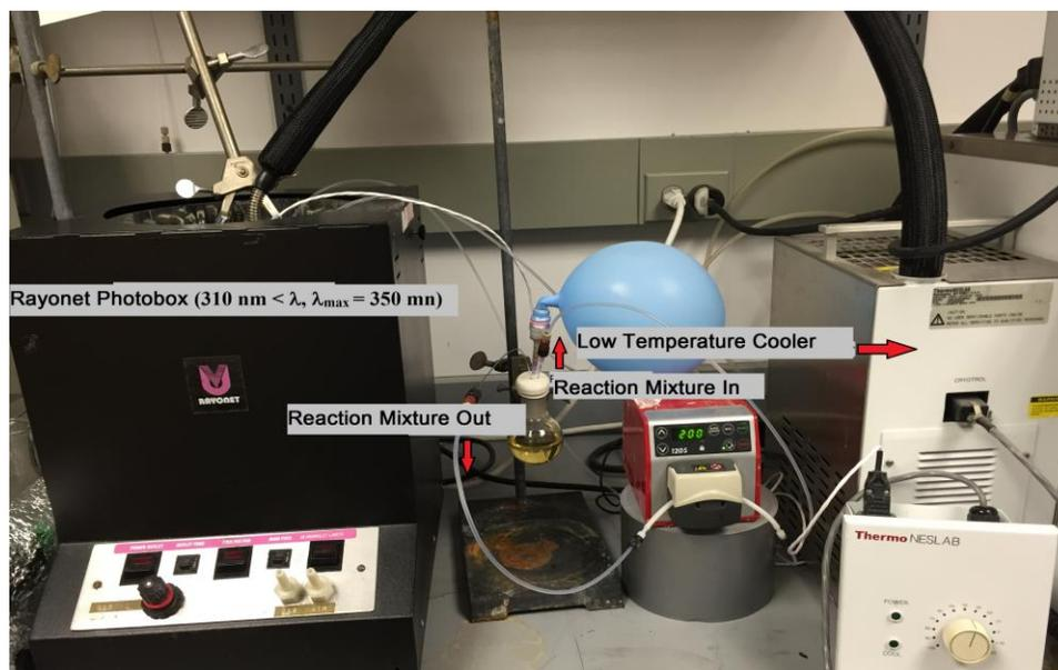
Figure SI-1b. Solvent Pumping System
