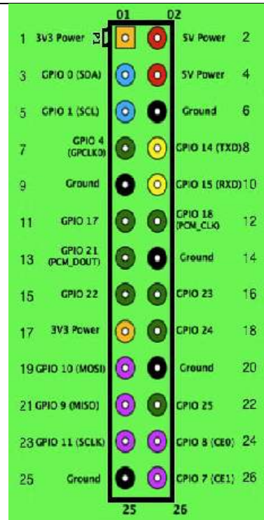
Figure 2: Raspberry Pi GPIO pins scheme
