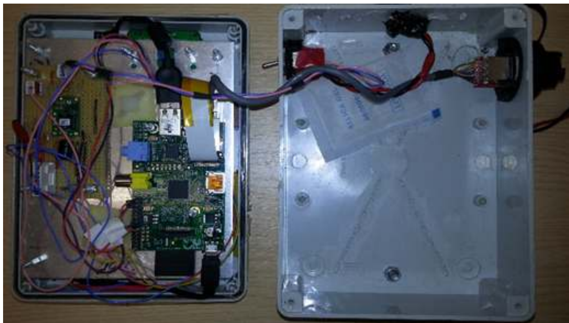
Figure 8: Inside view of WiseEye. The waterproof box has dimensions of 150 x 200 x 80 mm
