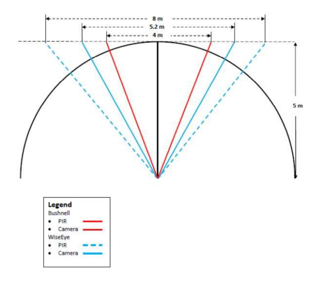
**S1 Fig. Comparison of field of view of the PIR sensor and camera for the WiseEye and Bushnell camera traps.** The detection zone and camera field of view of the Bushnell are the same. For reference the thick black line shows the 5 m radius.
