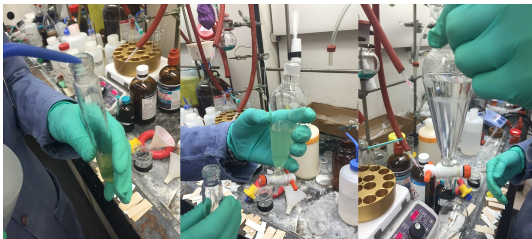
(Left) Dilution with \text{Et}_2\text{O} . (Center) Transfer to a separatory funnel. (Right) 0.1 M HCl wash.
