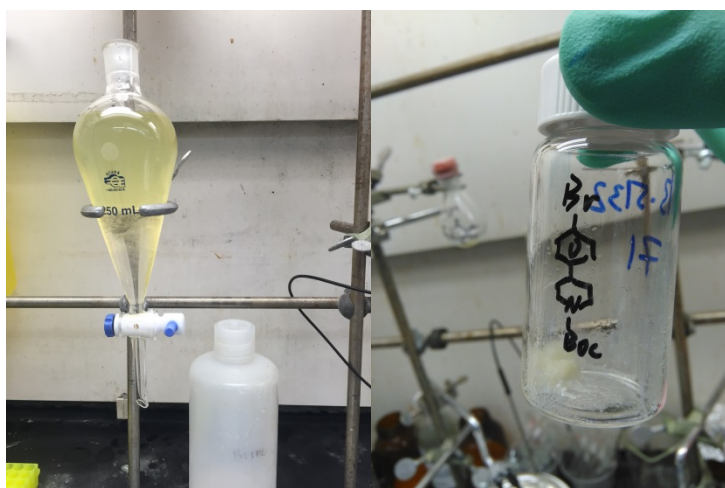
(Left) Wash with brine. (Right) Pure product after flash column chromatography.
