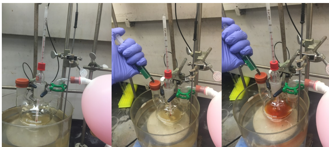
(Left) Internal temperature reached 75\text{ }^\circ\text{C} indicated by thermometer. (Center) Adding Ni/ligand complex (0.05 M in DMF, 10.0 mL, 20 mol%). (Right) Reaction mixture immediately turned red after first drop of Ni/ligand complex.
