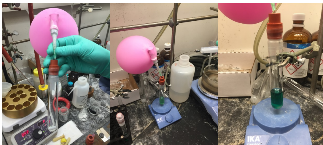
(Left) The flask with a stir bar was sealed with a septum, wrapped with parafilm, evacuated under vacuum and refilled with argon. This was done 3 times in total. (Center) Add DMF (6 mL) into the vial. (Right) After stirring for 3 hours at room temperature.
