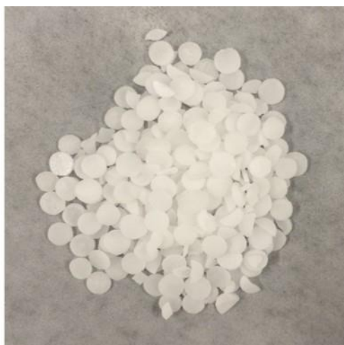
fig. S2. A digital photograph showing that the TPP molecules are flake-like crystals.
