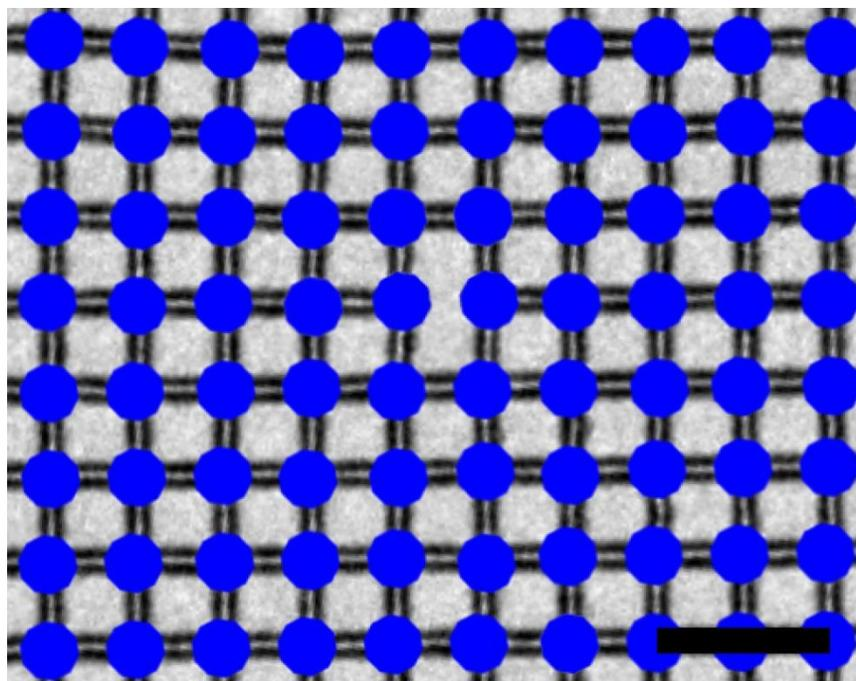
**Supplementary Figure 1 | Vertex map of a non-topological defect.** A simple vacancy, a single missing spin in an otherwise perfect square lattice, does not nucleate a vertex chain or result in topological frustration. Long range ground state ordering is not affected by the presence of a vacancy since it is not a topological defect. Scale bar is 1  $\mu\text{m}$ .
