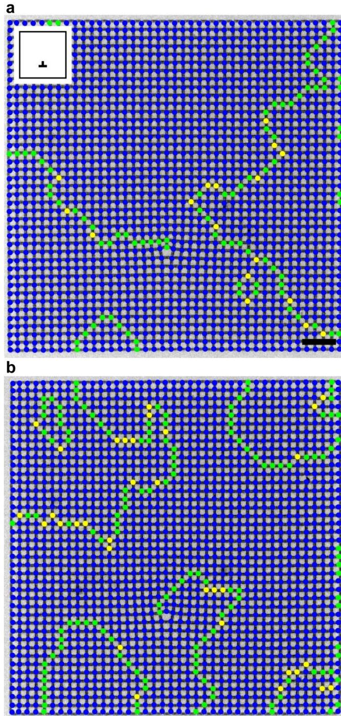
**Supplementary Figure 2 | Repeated annealing of the same crystal.** The same crystal is annealed twice under the same conditions and results in different domain configurations. The quenched disorder in the sample gives qualitatively similar, but not exactly reproducible ordering of vertices.
