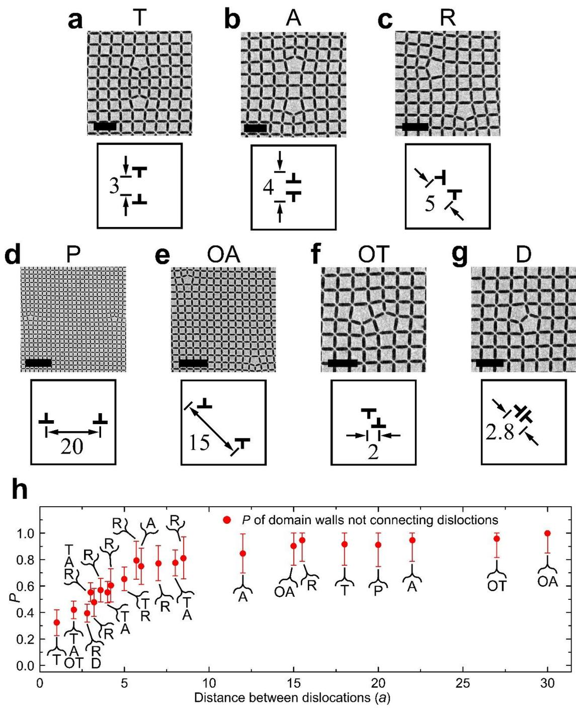
**Supplementary Figure 3 | Geometries studied.** (a-g) Definitions for families of two-dislocation geometries studied in this work. Each frame describes one family of geometries where the spacing between dislocations is varied. The spacing is given in units of the lattice constant ( $a \approx 500$  nm).
