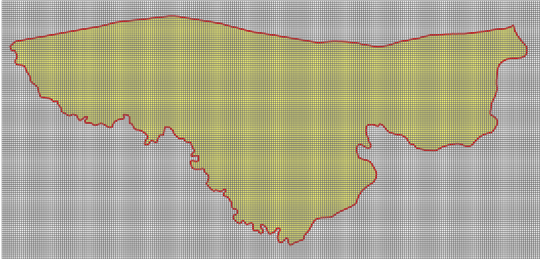
Figure S15. Grid used in the groundwater flow simulation. Map was created using ArcGIS 9.3 ( http://www.esri.com/software/arcgis/arcgis-for-desktop ).
