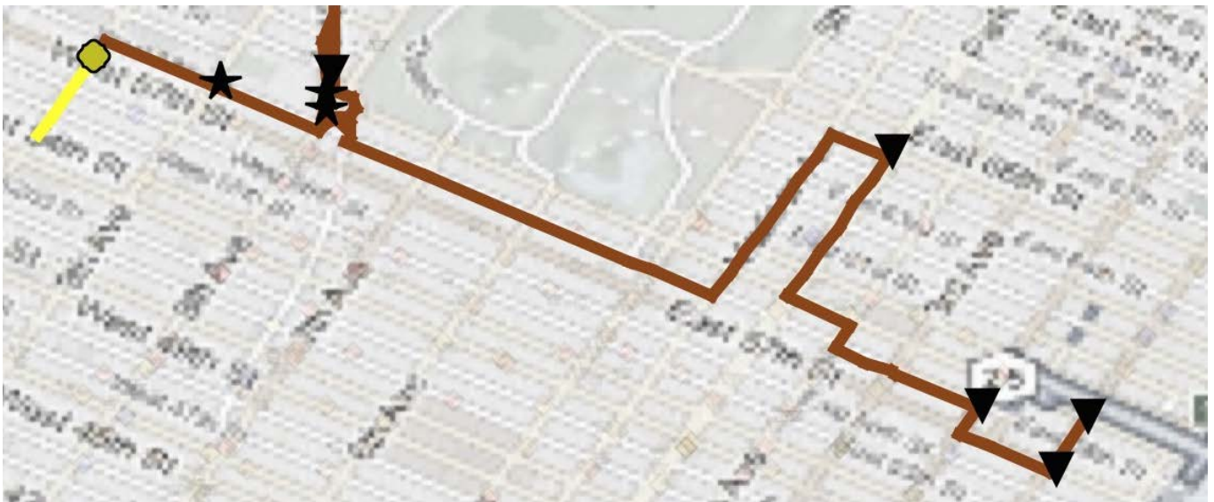
Fig. 2. Past path (yellow) and optimal path (brown) for a vehicle (yellow dot) with two passengers and scheduled pick up of three requests (star) and drop-offs (triangle).
