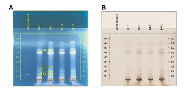
**Figure S1. HPTLC.** HPTLC image graphs of the extract samples. Graph A is measured at the wavelength 366 nm and B is the same graph under white RT light. BP means the extraction method is followed by British Pharmacopoeia. Two replications of each extract samples. The Rf value represents 0.09 (Withaferin A), 0.014 (Standard/Withanolide A) 0.24 (Withanolide B), 0.6 (β-sitosteol).
