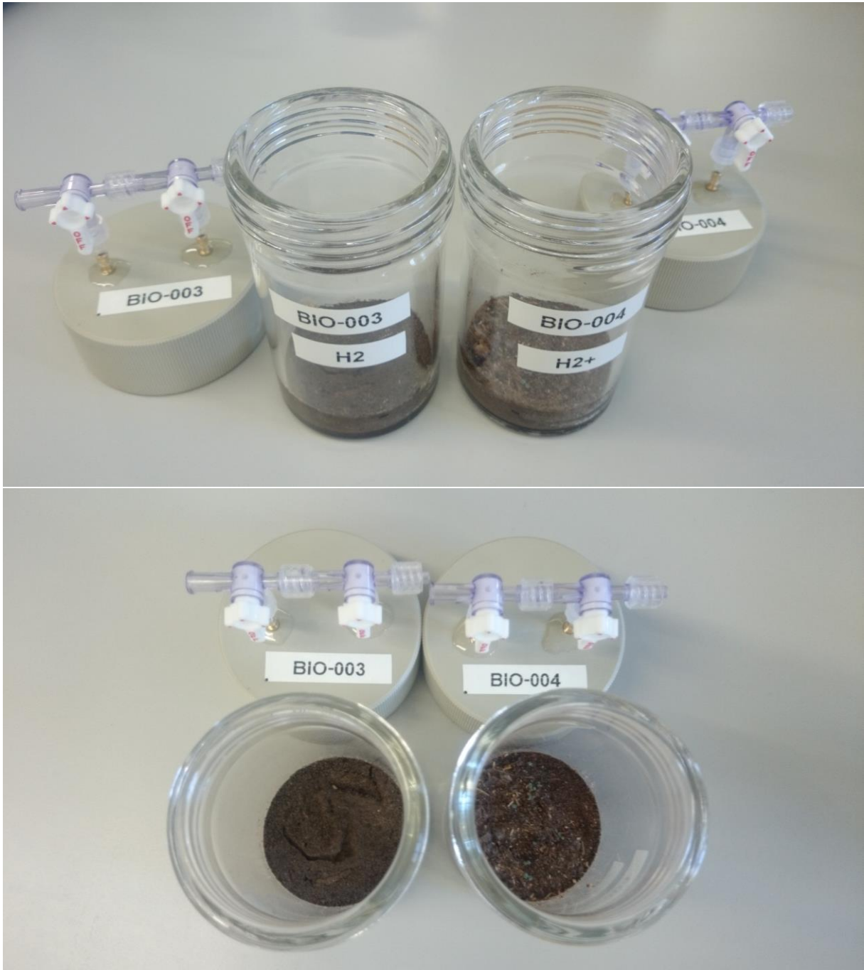
Fig. 4. Jars with experimental soils (40 g of soil, moisturized to a water filled pore space of 60% and set to a bulk density of 1.5 g/cm 3 ) without litter (left) and with litter (right). The amount of litter (mass, in gram per cm 2 in the jar) is proportional to the available litter in the forest stand (gram per m 2 in the forest).
