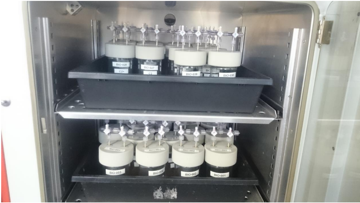
Fig. 2. The jars with moisturized soils (water filled pore space = 60%) are incubated for 12 days at 25°C. Valves are opened (levers are up) (2.6, 2.6.1).
