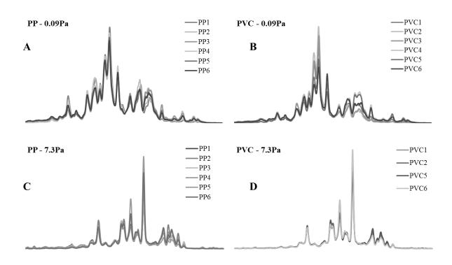
The repeatability for the bacterial communities was also investigated. Six slides of each material placed under the same shear stress were analyzed with the CE-SSCP fingerprinting technique. For each graph, SSCP profiles overlaid very well, highlighting a good repeatability for both materials and shear.
