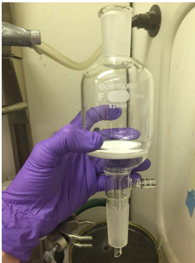
Figure S1. 150-mL ChemGlass Filtration Büchner Funnel with a 24/40 Joint
