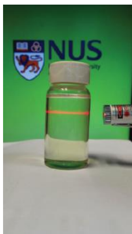
Supplementary Figure 5 | Tyndall effect of MAMS-1 nanosheets suspended in hexane.
