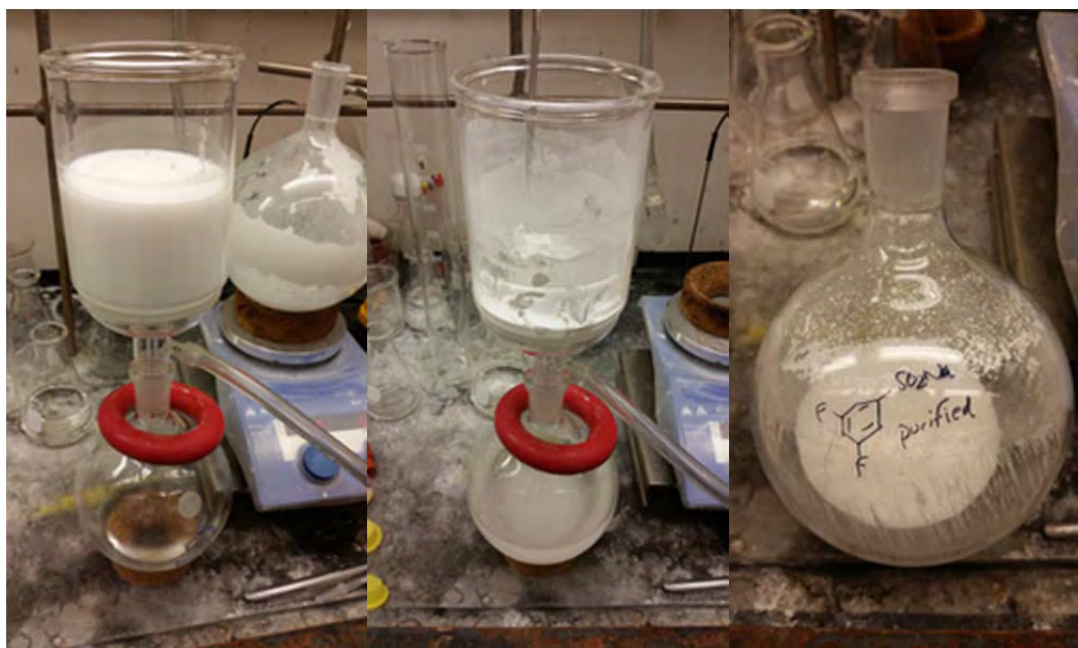
Fig. S77. Left. The crude sulfonate was treated with 500 mL of hot MeOH (twice) and filtered. Center. Cake of inorganic salts removed from sulfonate. Right. Purified sulfonate as a flowing white solid after concentration, azeotrope with toluene, and high vac.
