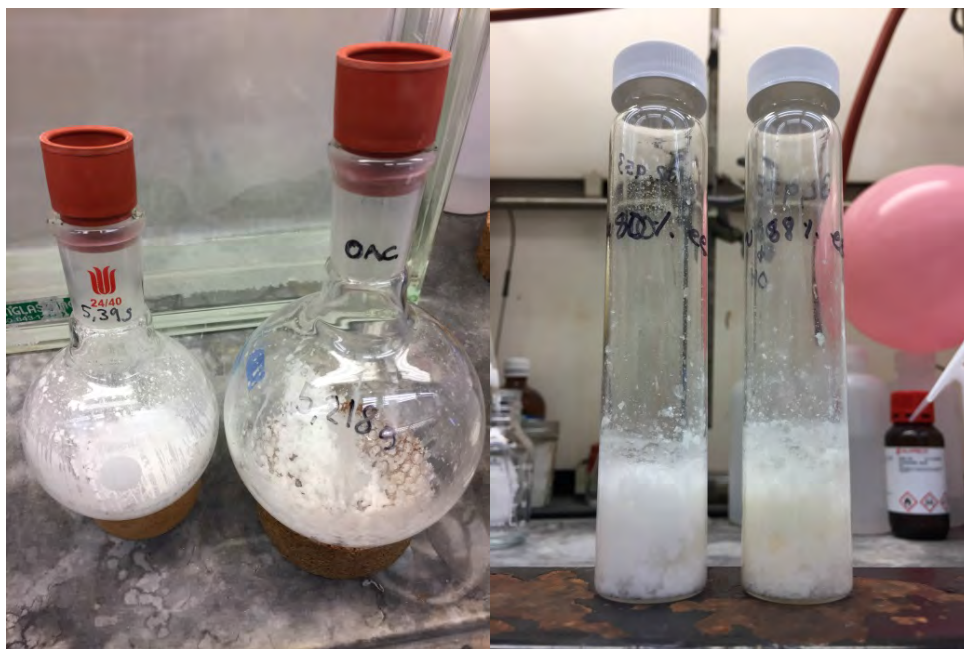
Fig. S109. Left. The alcohol 167a and acetate 169 were readily separated using silica gel chromatography. The acetate is then directly dissolved in MeOH and deacetylated using Na(s). Right. The resolved alcohol starting material ( left vial ) and deacetylated product after aqueous work-up ( right vial ).
