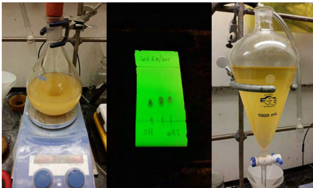
Fig. S90. Left. The reaction was allowed to warm to room temperature overnight (solution became yellow). Center. TLC conditions – 50% EtOAc in hexanes; left lane – crude alcohol; center lane – co-spot; right – reaction mixture. Right. H 2 O was added to the reaction mixture, the layers separated and the organic layer dried over Na 2 SO 4 .
