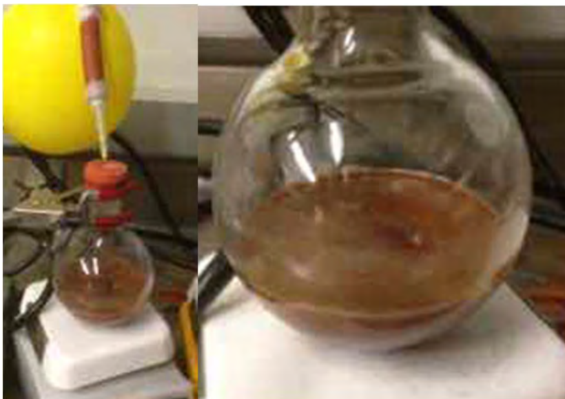
Fig. S17. Left. After stirring for 2h, the suspension turns a dark brown color. Right. Close up view of the suspension.
