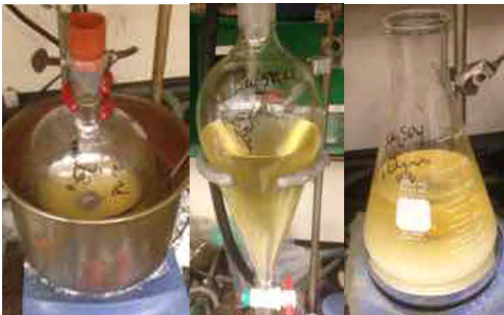
Fig. S31. Left. The reaction was heated at 60 °C for 2h. Center. The reaction was diluted with EtOAc and H 2 O. The organic layers were combined and washed with 5% aqueous LiCl. Right. The combined organics were dried over Na 2 SO 4 .
