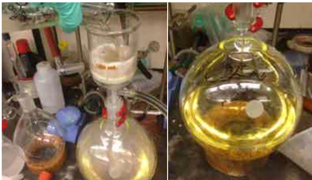
Fig. S32. Left. The combined organics were passed over silica. Right. The crude material was collected in a single flask and used in the next reaction without further purification.
