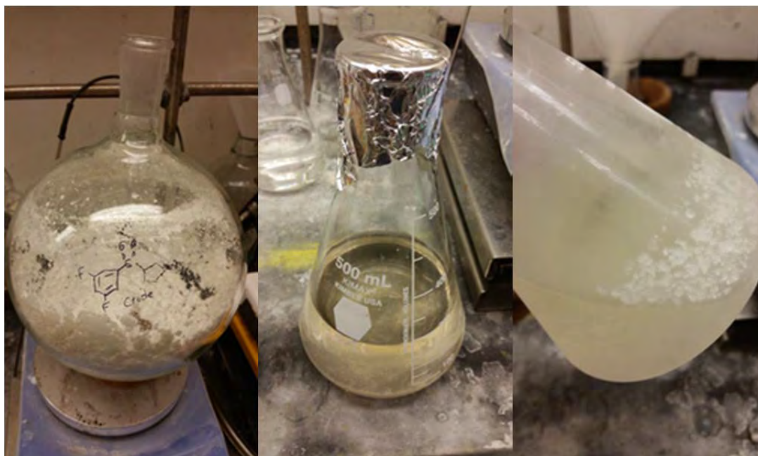
Fig. S82. Left. The ketone was azeotroped with toluene and could be used in the next reaction without further purification. Center. If desired, the ketone could be recrystallized from \text{CH}_2\text{Cl}_2 . Right. Crystals form after slow cooling to -20\text{ }^\circ\text{C} .
