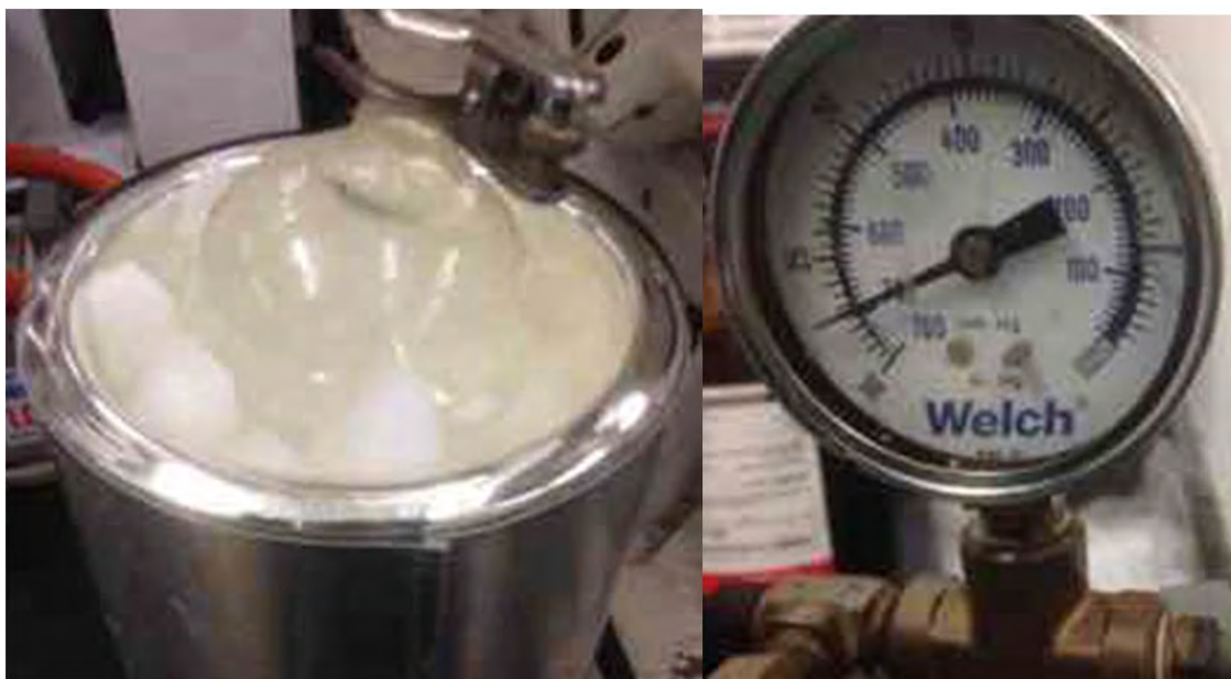
Fig. S19. Left. The receiving flash is immersed in a dry ice/acetone bath at -78\text{ }^{\circ}\text{C} . Right. The pressure of the distillation is carefully controlled beginning at ca. 10 Torr.
