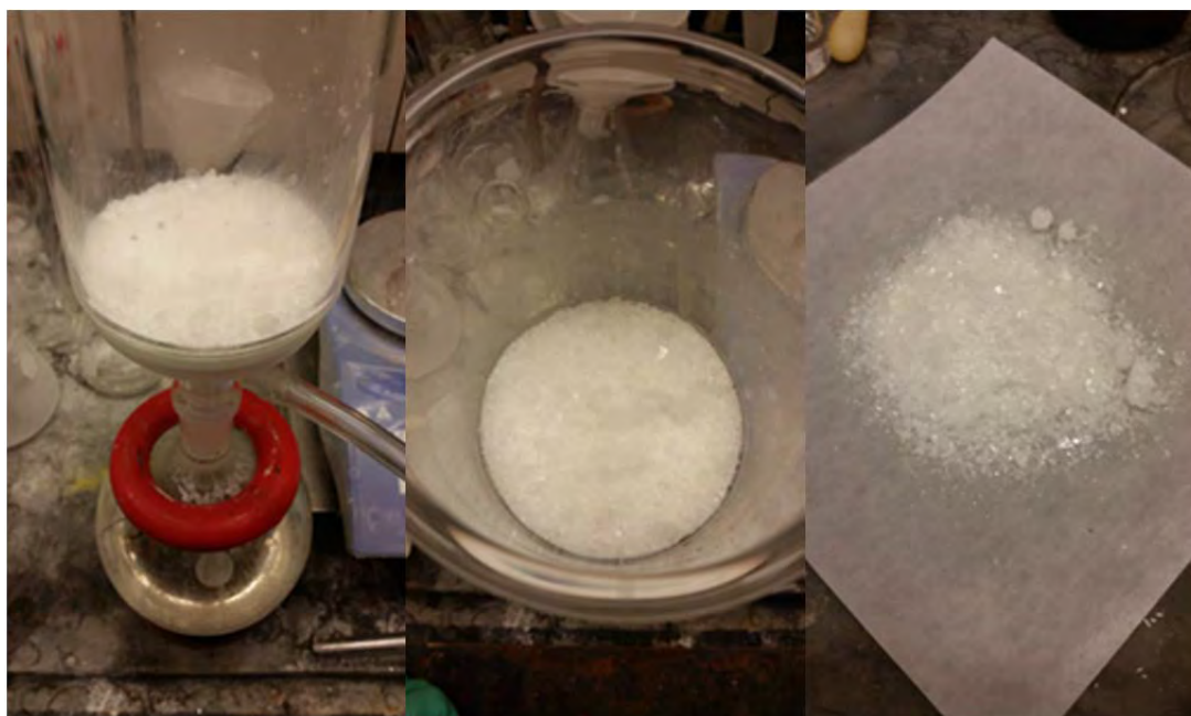
Fig. S83. Left. The crystals were collected by filtration. Center. The crystals were washed with a small portion of ice cold \text{CH}_2\text{Cl}_2 . Right. Recrystallized ketone.
