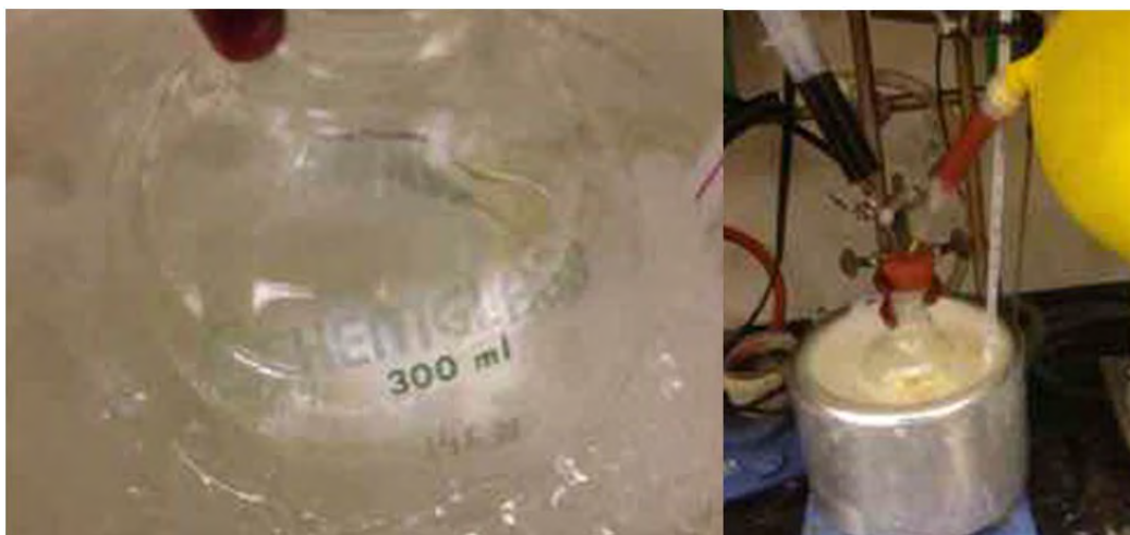
Fig. S14. Left. To consistently maintain -45\text{ }^{\circ}\text{C} for ca. 20 minutes, the dry ice should be dissolved in isopropanol. The bath should appear homogeneous and not contain any solid pieces of dry ice. Right. Addition of PhLi at -45\text{ }^{\circ}\text{C} .
