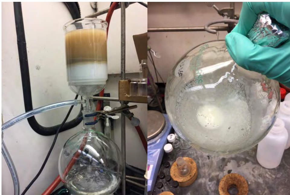
Fig. S108. Left. The reaction is stopped by passing the reaction mixture through a short plug of \text{SiO}_2 on a frit funnel. Additional EtOAc is added to pull material through the plug. Subsequently, all volatiles including excess vinyl acetate are removed on a rotary evaporator. Right. Concentrated reaction mixture after filtration.
