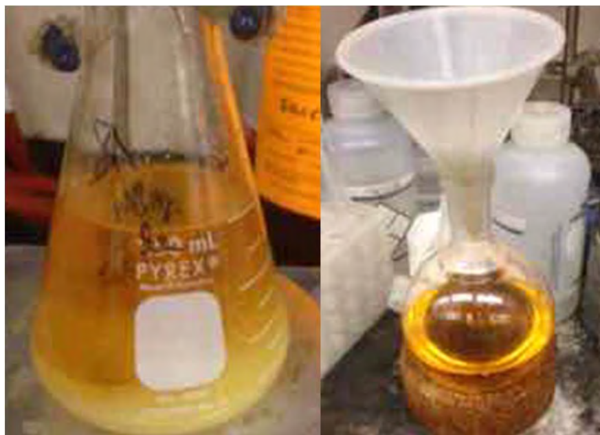
Fig. S10. Left. The combined organics are dried over \text{Na}_2\text{SO}_4 . Right. The combined organics are filtered through cotton and concentrated in vacuo .
