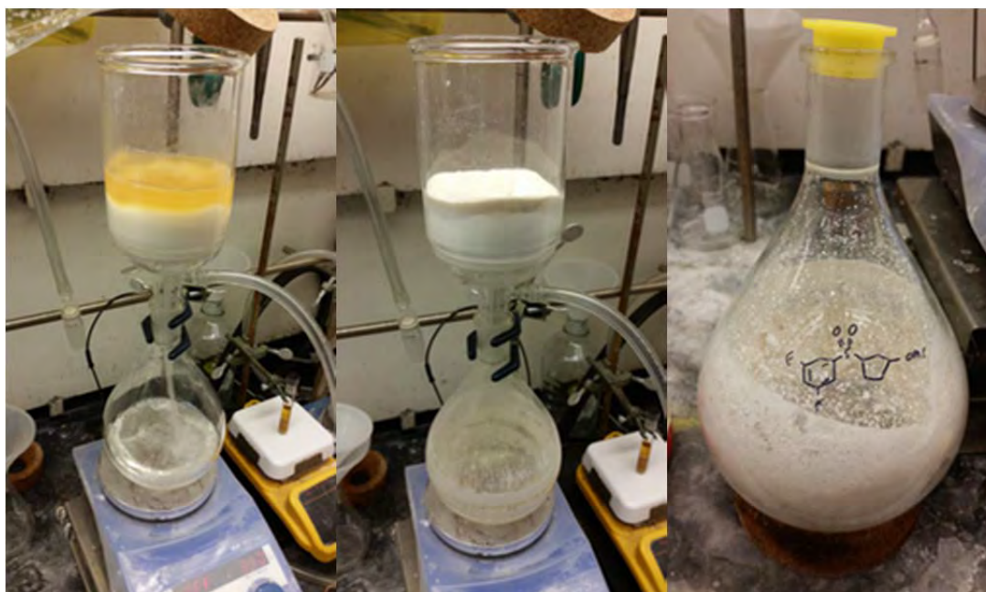
Fig. S91. Left. The dried, combined organic layers were passed over a short pad of silica gel. Center. The pad was washed with 15% EtOAc in CH 2 Cl 2 (200 mL). Right. The extracts were concentrated to a white solid.
