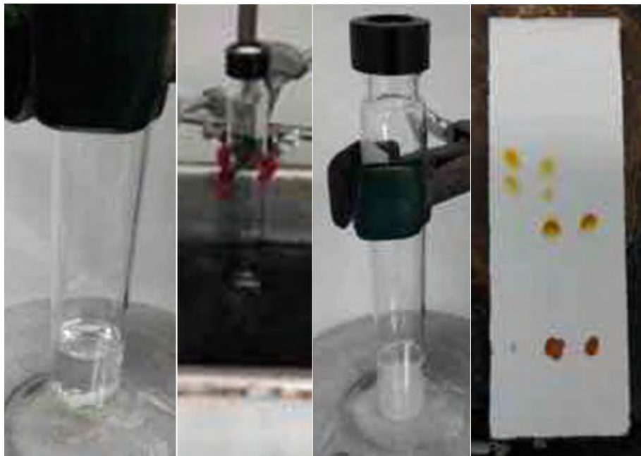
Fig. S54. Left. Aminated sulfone intermediate of 134 dissolved in MeOH with activated Mg turnings added. Left-Center. Sonication of reaction for 5 min. Right-Center. Reaction after stirring with MeOH/Mg until completion. Right. TLC with I 2 development (1:6 MeOH:CH 2 Cl 2 ). Lane 1 = nortriptyline cyclobutylsulfone; Lane 2 = co-spot of nortriptyline cyclobutylsulfone and crude reaction mixture; Lane 3 = crude reaction mixture.
