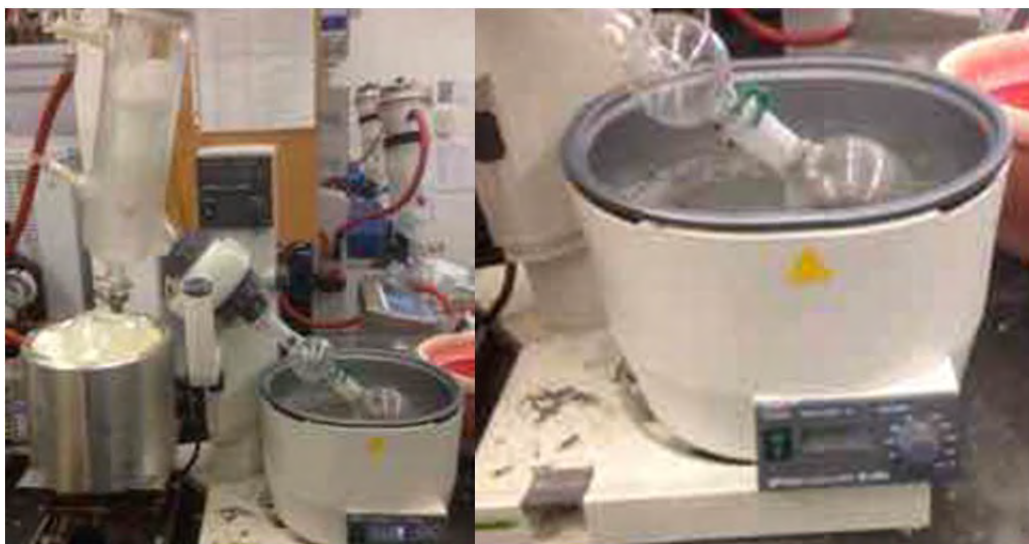
Fig. S18. Left. The suspension is distilled directly on the rotovap. Right. The water bath is maintained at ca. 20 °C during the course of the distillation.
