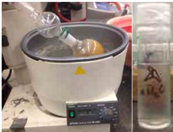
Fig. S21. Left. View of the reaction flask at the end of distillation. Do not distill to dryness ; the flask should contain a suspension of salts in \text{Bu}_2\text{O} . Right. Stock solution of [1.1.1]propellane in diethyl ether.
