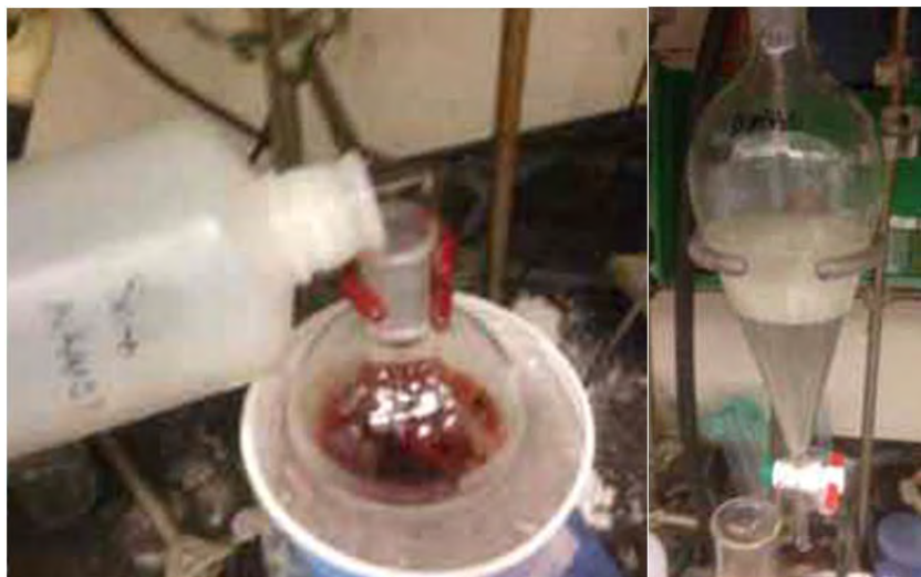
Fig. S43. Left. The reaction was quenched with sat. aq. \text{NH}_4\text{Cl} and extracted with \text{CH}_2\text{Cl}_2 . Right. The aqueous layer was extracted with \text{CH}_2\text{Cl}_2 (note: thick emulsion in aqueous layer).
