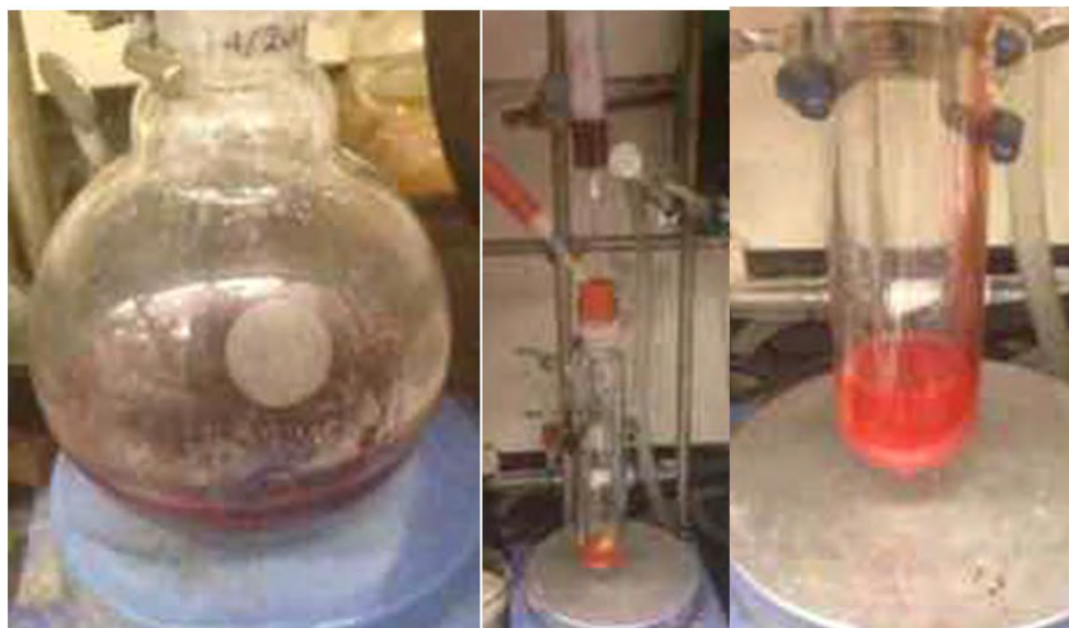
Fig. S6. Left. Flask of the “turbo amide” solution (ready to be used). Center. Upon addition of the “turbo amide” the color of the reaction mixture changes from yellow to orange/red. Right. Close up of the reaction mixture after the addition of the “turbo amide.”
