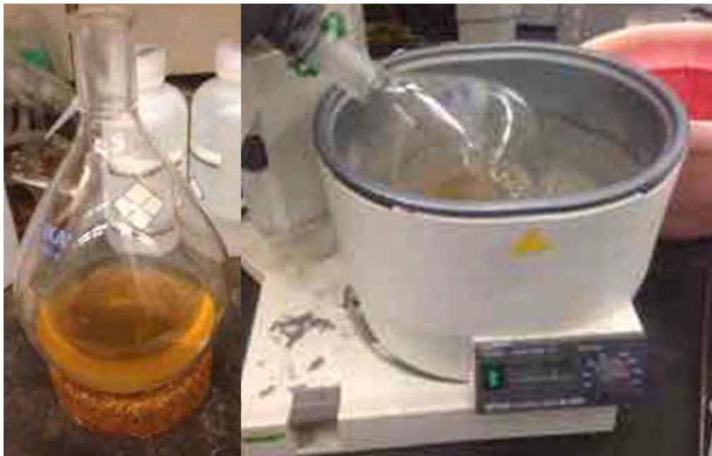
Fig. S27. Left. Conversion of 3,5-difluorobenzenesulfonyl chloride to sodium 3,5-difluorobenzenesulfinate after heating at 80 °C for 16 h. Right. The crude product was azeotroped with toluene to remove residual H 2 O.
