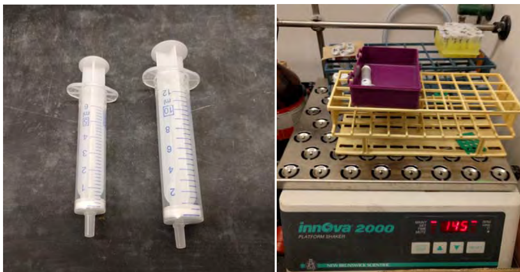
(Left) Solid-phase reaction vessels purchased from Torviq. (Right) Orbital shaker for solid-phase peptide synthesis (SPPS).
