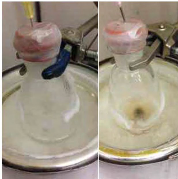
Fig. S23. Left. Suspension of 87 in dry THF is cooled to -78\text{ }^{\circ}\text{C} . Right. After addition of PhLi, the color changes from colorless/white to pale yellow.
