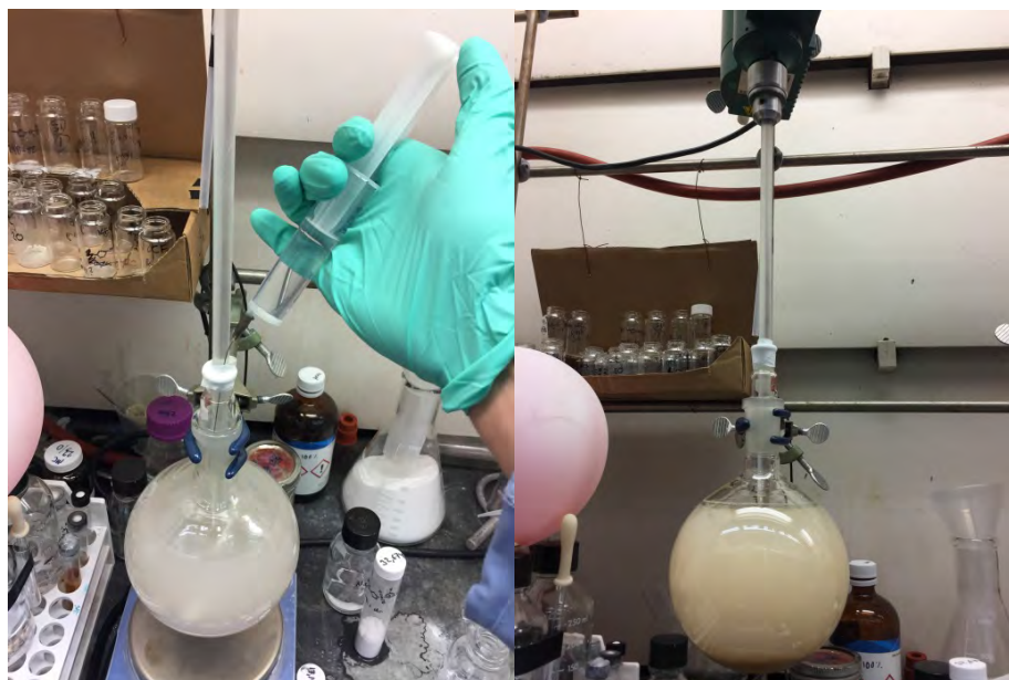
Fig. S107. Left. Addition of vinyl acetate by syringe. Teflon tape is wrapped around the flask's neck to suppress solvent evaporation. Right. The reaction mixture after 12 h stirring.
