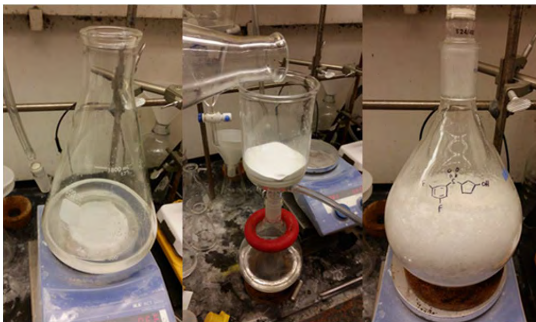
Fig. S87. Left. The combined organic layers were dried over \text{Na}_2\text{SO}_4 . Center. The dried, combined organic layers were passed over a short pad of silica gel. Right. The solvent was removed in vacuo to give the crude alcohol as a white solid.
