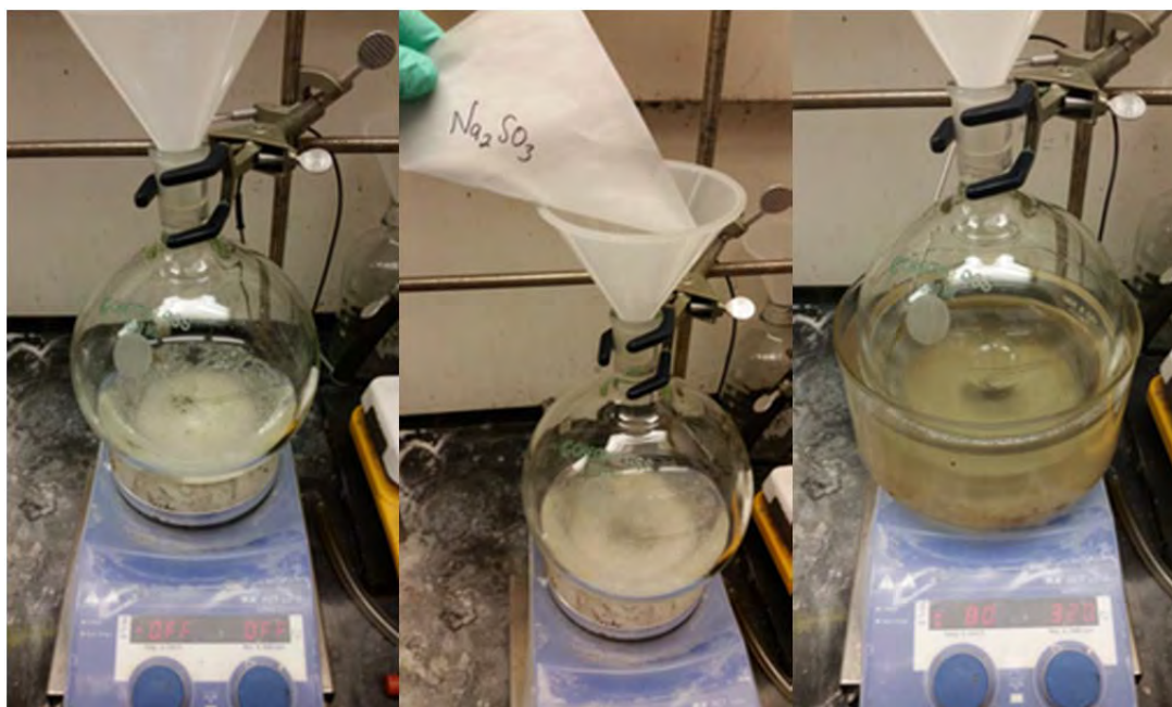
Fig. S74. Left. The sulfonyl chloride was suspended in \text{H}_2\text{O} . Center. Sodium sulfite was added. Right. The suspension was heated to 80\text{ }^\circ\text{C} and became a clear solution.
