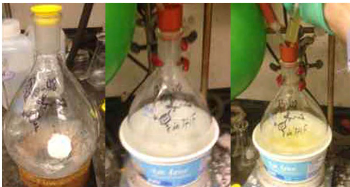
Fig. S36. Left. Pure epoxide (white solid). Center. The epoxide was dissolved in THF and cooled to 0 °C. Right. n -BuLi was slowly added to the reaction mixture.
