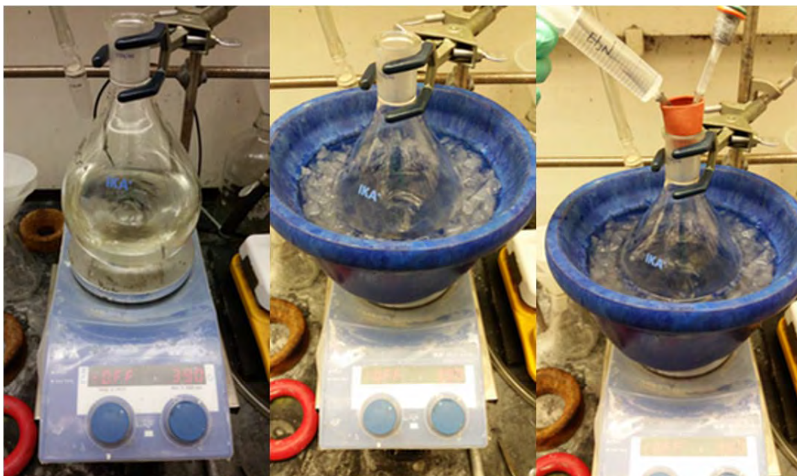
Fig. S88. Left. The crude alcohol was dissolved in \text{CH}_2\text{Cl}_2 . Center. The solution was cooled to 0\text{ }^\circ\text{C} in an ice-water bath. Right. Triethylamine was added via syringe (slow stream for addition, not dropwise).
