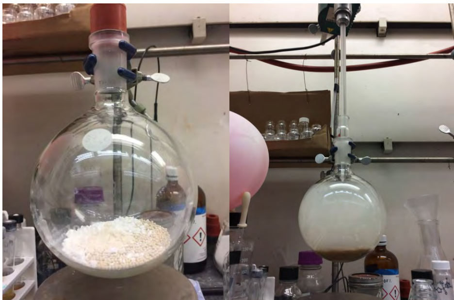
Fig. S106. Left. Addition of 167 (10 g), lipase, and molecular sieves in an oven-dried round-bottom flask. Right. Addition of MTBE (800 mL) and attachment of mechanical stirrer
