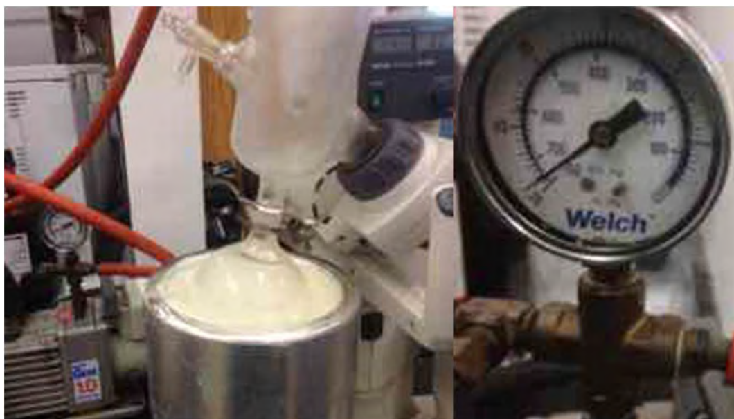
Fig. S20. Left. View of the distillation in progress. Right. The pressure is reduced to ca. 4 Torr to complete the distillation.
