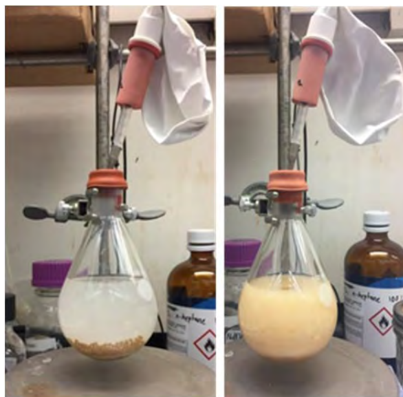
Fig. S100. Graphical presentation of kinetic resolution of 100 mg 167 . Left. 0 h; Right. 48 h. The empty balloon is attached in order to accommodate potential build-up of gas.
