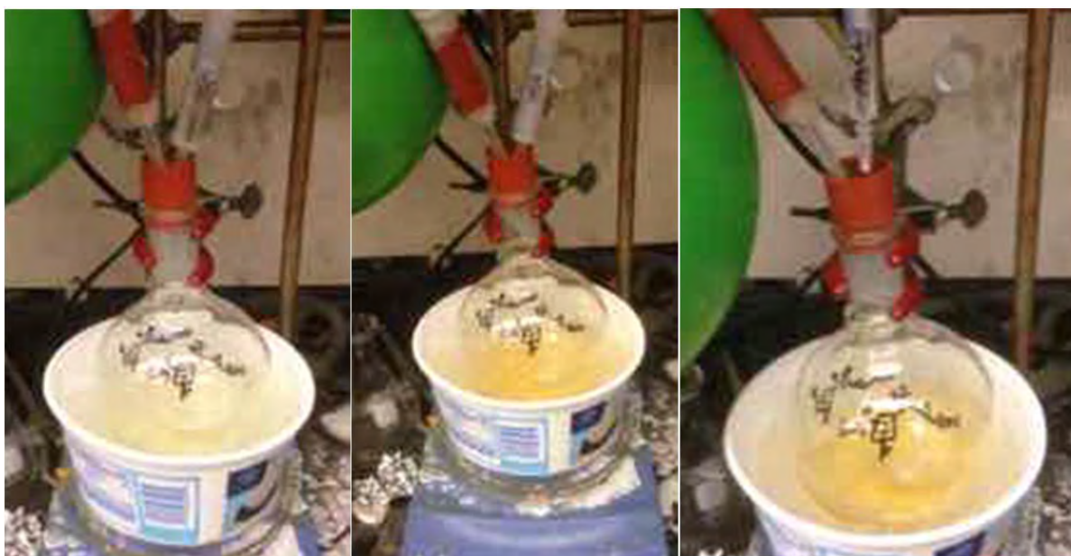
Fig. S39. Left. The crude alcohol was dissolved in \text{CH}_2\text{Cl}_2 and cooled to 0\text{ }^\circ\text{C} . Center. \text{Et}_3\text{N} was added. Right. Methanesulfonyl chloride was added.
