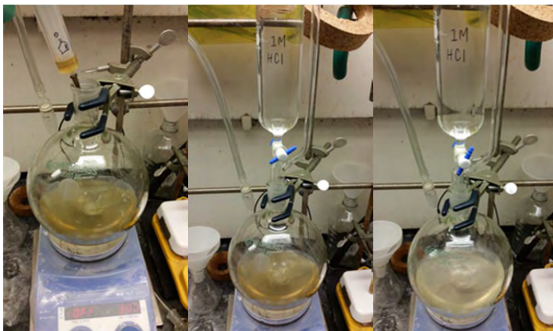
Fig. S79. Left. The reaction became yellow with the addition of 162 . Center. The flask was fitted with an addition funnel containing 1M HCl. Right. During the initial addition of the HCl, the reaction turned from yellow to colorless.
