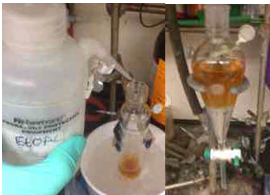
Fig. S9. Left. The quenched reaction mixture is diluted with EtOAc. Right. The solution is transferred to a separatory funnel and the organics washed with \text{H}_2\text{O} .
