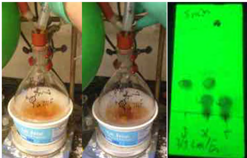
Fig. S37. Left. During the addition of n -BuLi, the reaction turns orange. Center. By the end of the n -BuLi addition, the mixture turns red. Right. After 5 minutes, TLC shows complete consumption of the starting material. Lanes: Left = Starting epoxide; Center = Co-spot; Right = Crude reaction mixture (solvent system = 7:3 EtOAc:hexanes).
