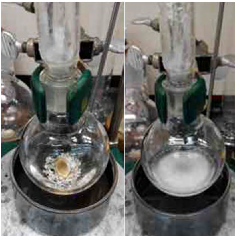
Fig. S52. Left. The crude product (same flask as rotovap) was dissolved in MeOH and activated Mg turnings added. Right. The Mg/MeOH reduction after heating at 80 °C for 2 h.
