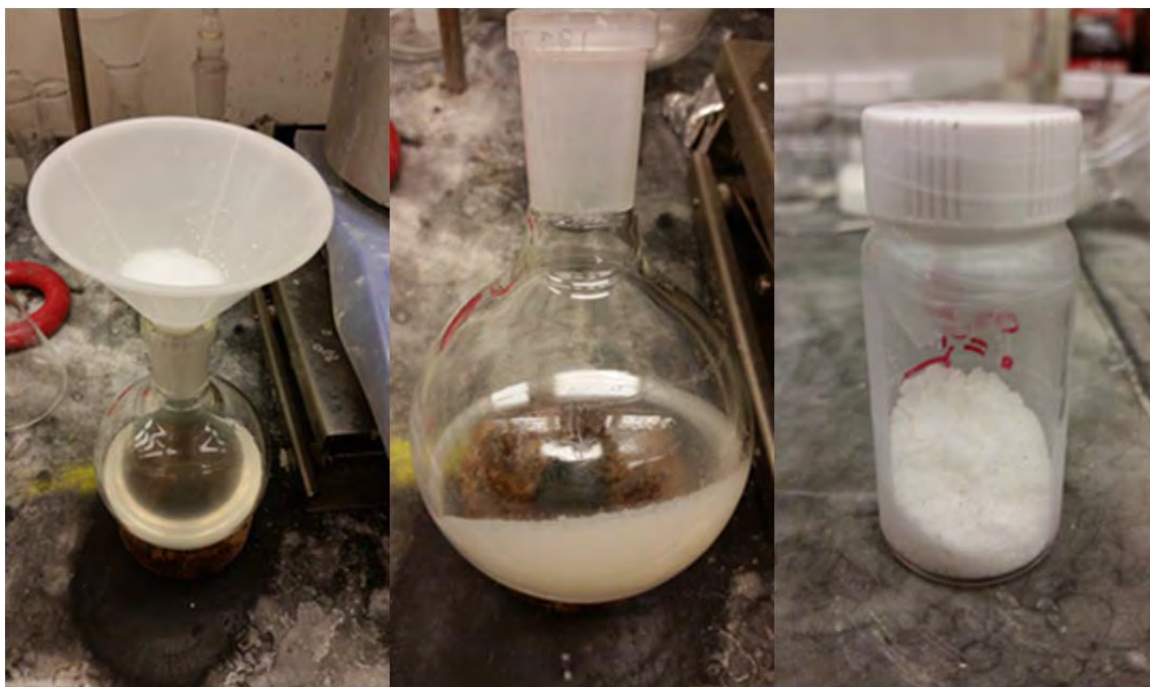
Fig. S95. Left. The dried, combined organic layers were filtered and concentrated. Center. Crude strain-release reagent 9 as a pale yellow solid. Right. Purification by flash chromatography (0 to 20% EtOAc in hexanes) gave 9 as a white crystalline solid.
