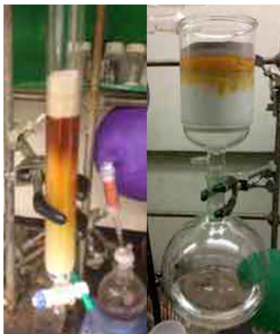
Fig. S11. Left. The crude material is wet loaded onto silica (ca. 20 g) and eluted in a single flask (no fractions) with 0 to 3% EtOAc in hexanes. Right. Alternatively, the crude material was dry loaded onto a silica pad in a sintered glass funnel and eluted in a single flask (no fractions) with 0 to 3% EtOAc in hexanes. Note: this picture is from a 10 g scale run.
