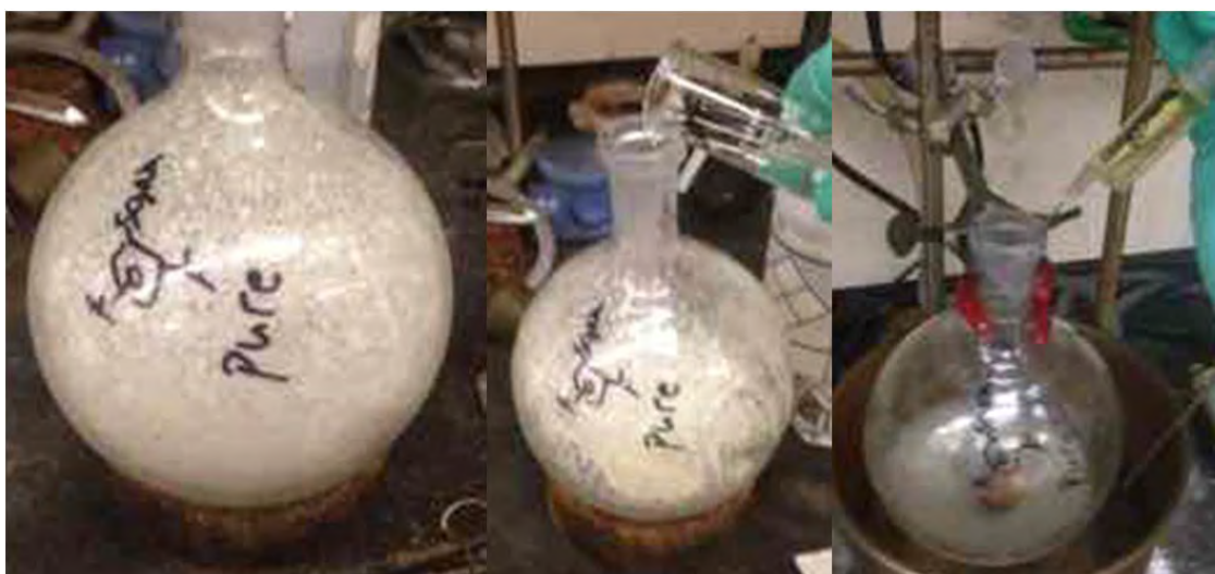
Fig. S30. Left. Purified sodium 3,5-difluorobenzenesulfinate was transferred to a round bottom flask. Center. DMF was added. Right. 4-Bromobut-1-ene was added.
