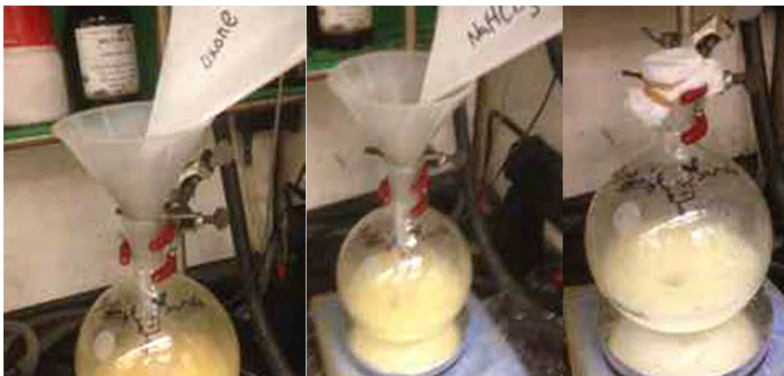
Fig. S33. Left. The crude alkene was dissolved in 1:1 acetone and H 2 O. Oxone was added. Center. NaHCO 3 was added. Right. The mixture was stirred at room temperature for 20 h.
