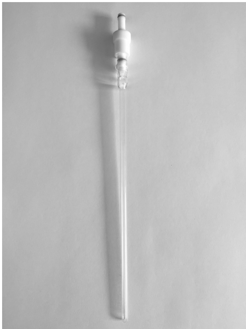
Figure S2. Modified 535PP 5 mm 600 MHz NMR tubes from Wilmad (Vineland, NJ) fused to CG-513 European style NMR tube valves purchased from Chemglass (Vineland, NJ) by Daryl Smith (Glassblower, Yale Chemistry Department).
