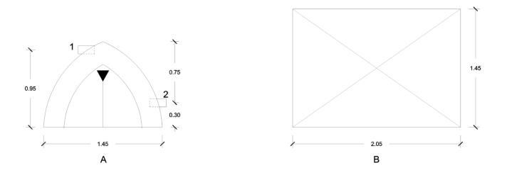
(A) Front view – 1) device for the exiting of air (screened 1-m PVC tube); 2) device for the entry of air (screened 1-m PVC tube) with cooler (not shown in figure) to adjust velocity; (B) Schematic of tent.
