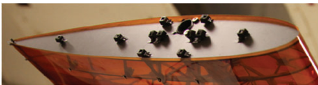
SUPPLEMENTARY FIG. S8. Wing boundary condition. Wing tip end cap with bolts to shaft collar, end of torque tube, and zip tie connection to lattice. The lattice acts as a continuous structure between these two boundaries, achieving load transfer and effecting actuation.
