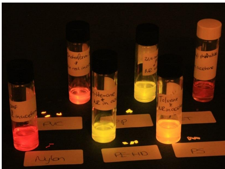
Fig S19. Polymers dyed with Nile Red, ( 1000 \mu\text{g mL}^{-1} in acetone). Polymers are placed adjacent to vials containing solvents of similar structure/polarity. Taken under blue light (Crime Lite: 450-510 nm) through an orange filter (529 nm).
