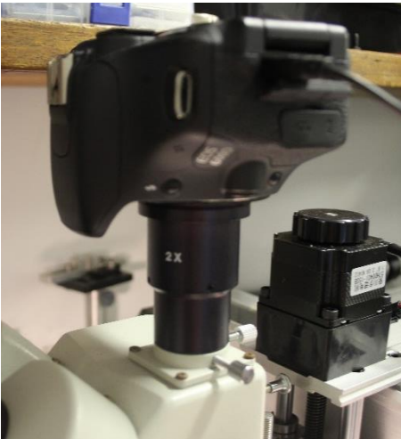
Fig S13. The mounting of the camera to the third port of the trinocular microscope head.
