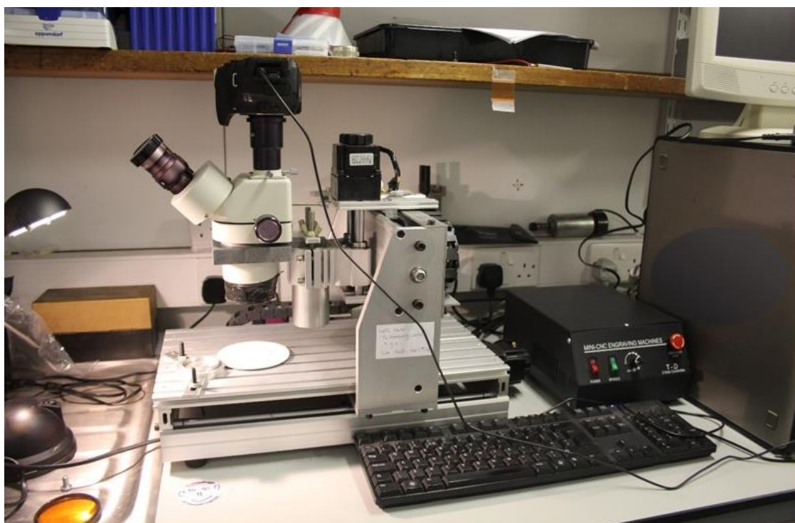
Fig S11. Overview of the imaging rig showing all the components for white light imaging. For fluorescence work, the orange filter (left bottom) would be taped below the microscope head and the blue crimelite would be substituted for the white light.
