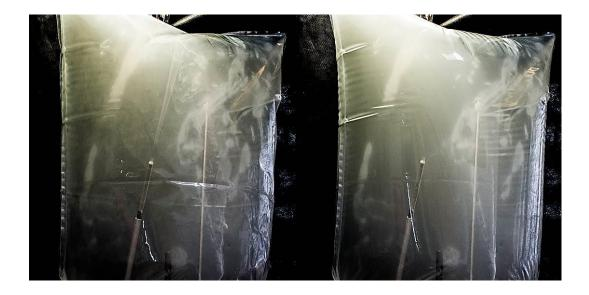
**Fig. S3 Gas mixing test.** Turbulent mixing within the chambers (left: no flow, right:  $10 l_n min^{-1}$ ). Black background and upward light installed to improve visibility (see video is available in Additional file 2). White areas in the left chamber represent the highly concentrated sulfuric acid particles leaving the smoke tube.
