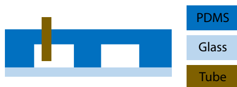
Fig. S1: The simple fabrication process for our device uses a standard soft-lithography process with only one lithography step. We use a 2 \mu\text{m} layer of SU-8 to improve the adhesion of small structures to the wafer. Here we show a cross-section of the final structure (not to scale).
