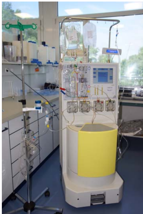
Figure 4: Photo of the IgE adsorber with the plasma separation unit COM.TEC
