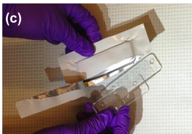
fig. S2. Vacuum charging and long-term storage. (a) After the chips are incubated in vacuum overnight (-95 kPa), it is sealed in an aluminum pouch with a vacuum sealer. It takes only several seconds to seal each pouch. There is a layer of plastic laminated on the inside of the aluminum seals, and by heating the seams up, the vacuum sealer can melt and seal the pouch. (b) Zoom in on the sealed pouch. This pouch can be stored indefinitely and transported easily to remote areas. (c) The user simply rips the seal open and load samples in. (d) Loading of the samples (food dye). With the vacuum battery system, there is a long operation window of ~2.5 hours for the user to load the chip.
