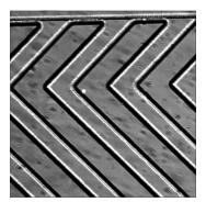
Supplementary Movie S2: Fluorescently labeled plasma cells spiked in healthy whole blood sample introduced into the herringbone microfluidic channel after Ficoll fractionation. The video is showing one captured plasma cell and other blood cells going with the flow.
