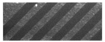
Supplementary Movie S3: Fluorescently labeled plasma cells spiked in unprocessed healthy whole blood sample introduced into the herringbone microfluidic channel. The video is showing a captured plasma cell and another one going with the flow. Red blood cells represent the major population of the unprocessed blood sample and shown to cause the cloudiness in the video.
