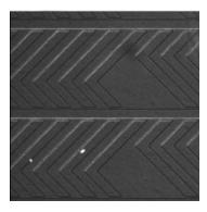
Supplementary Movie S1: Fluorescently labeled plasma cells spiked in PBS introduced into the herringbone microfluidic channel. The video is showing one captured cell and one cell flowing and changing its xyz coordinates because of mixing induced by the herringbone geometry.
