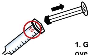
1. Get a stopwatch and some 10 mL syringes: see specification over the page. Remove the plunger from one syringe & discard.
