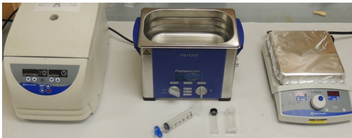
Figure SI-1. Only simple labware is required for the synthesis of the nanoshells. Left to right: Microcentrifuge, ultrasonic bath, 0.22 \mu\text{m} syringe filter, vials, stir bars and stirring plate.
