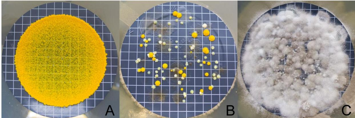
**Technical Appendix Figure.** Quantitative culture of filtered water from heater–cooler units. The images show filters with (A) >1,000 CFU/L, (B) 300 CFU/L with some contamination from other bacteria, and (C) heavy overgrowth of mold.
