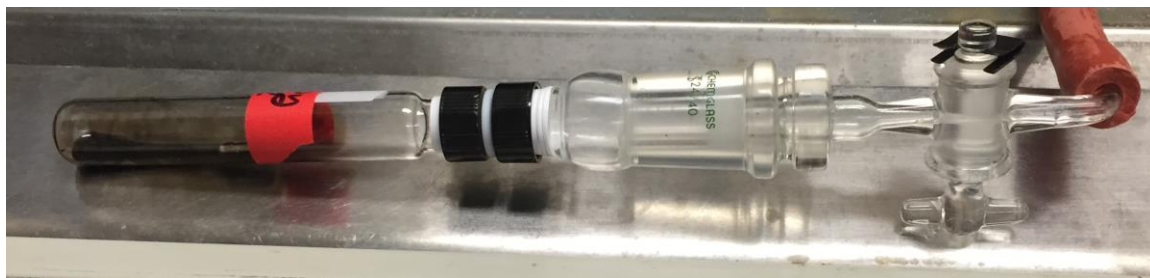
Figure SI-2: apparatus for solvent removal from the hydrosilylation mixture Procedure D.
