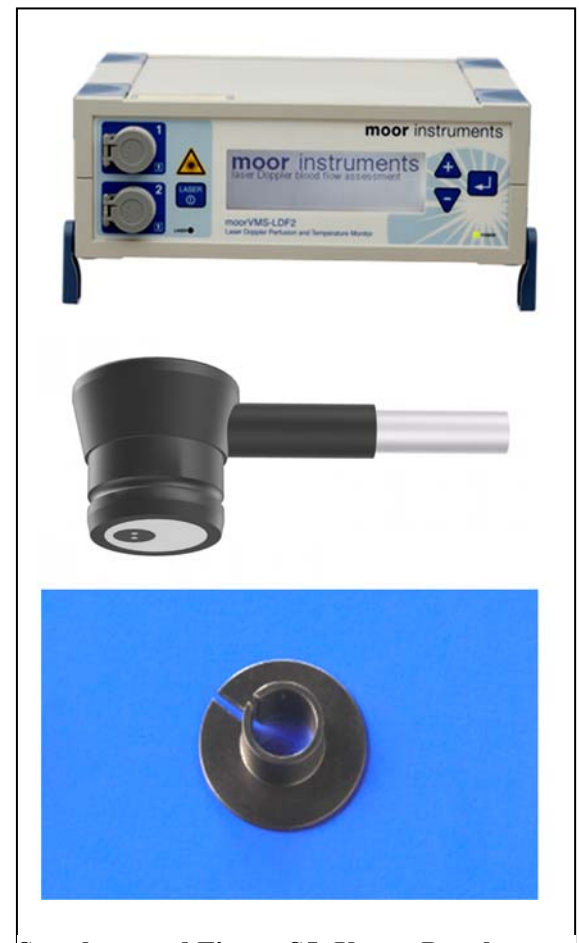
Supplemental Figure S5: Upper Panel: moorVMS-LDF™ monitor. The device comes with one or two-channel options. Multiple modules can be combined for a multi-channel system. Middle Panel: VP1T probe with emitting and receiving fibres incorporated into a single probe to minimize motion artifact. Each fiber is 0.5 mm in diameter and separated by 0.5mm. The probe has a height of 12.5mm (at the probe tip) and 8mm outside diameter. The groove around the tip of the probe allows the probe to clip into the probe holder. Lower panel: PH1-V2F probe holder.
