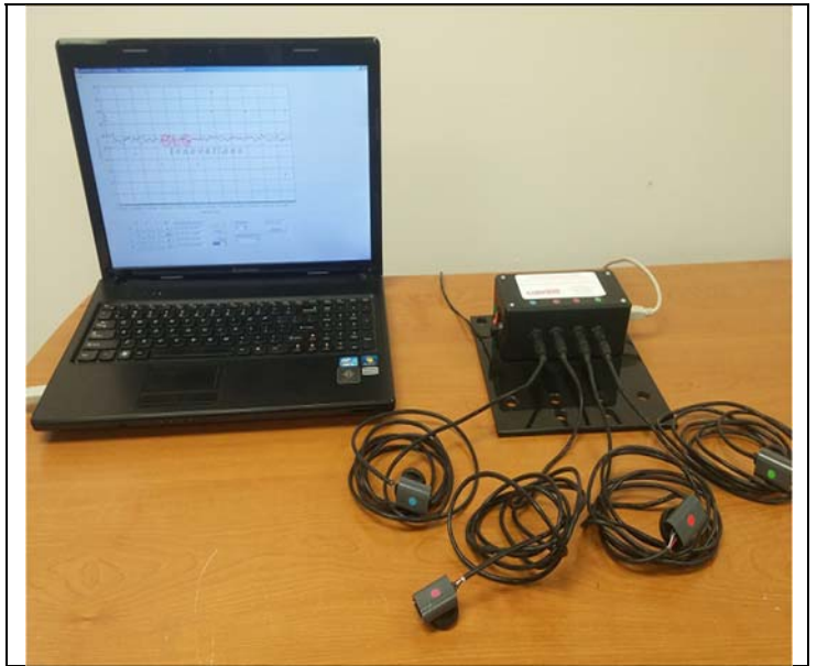
Supplemental Figure S3: cyberDERM clinical tristimulus colorimeter.
