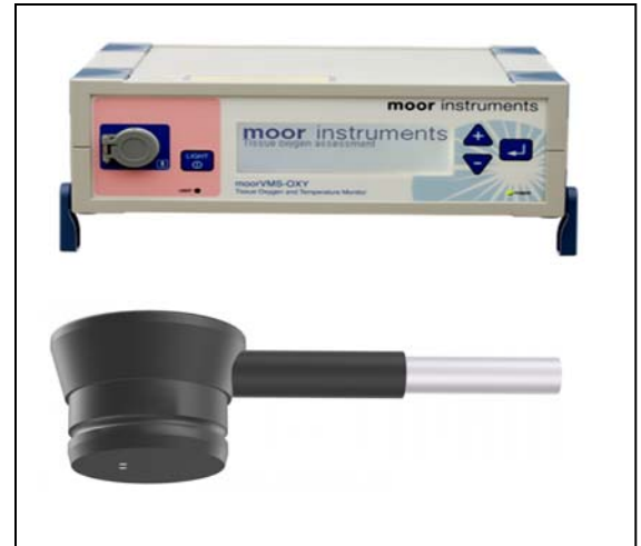
Supplemental Figure S4: Upper panel: moorVMS-OXY™ WLS device. Lower panel: Moor instruments OP1-1000 WLS probe. White light emitting and receiving fibres are separated by 1mm. The probe has the same dimensions as the LDF probe i.e 12.5 mm high and 8 mm outside diameter and uses the same probe holder as the LDF probe.
