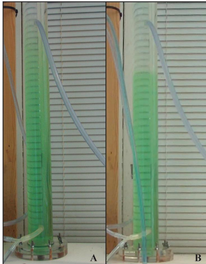
Supplementary Figure 2. Demonstration of the hydrodynamic conditions during the anoxic phase (with stained influent, and without sludge, for better visibility). Due to the plug-flow influent, the fresh wastewater remains at the bottom half of the reactor after feeding ( A , 5 min). The effect of diffusion dilutes the fresh influent, but the substrate concentration is still high at the end of the pre-anoxic phase ( B , 60 min). Green = fresh influent, colorless = residual liquid from the previous cycle. N.B. during the experiment, the stagnant sludge bed influenced the hydrodynamic conditions, e.g. the sludge partly displaced the influent due to the volume of the biomass and the volume of the residual liquid that fills the voids and pores of the granules.
