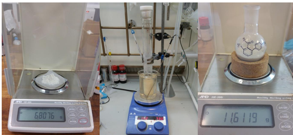
Figure 1. Left hand-side, o -toluic acid; centre, reaction mixture; right hand-side, pure 3aa .
