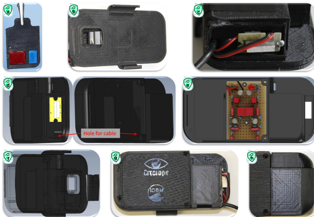
Fig. 15: Image-by-image instruction to build the smart phone add-on to measure algal fluorescence in water: How a) to glue the filter set up, b) to position the mirror, c) to fix the LED set up in to the 3D-element, d) to place the cables, e) to position the circuit board, f) to combine the smart phone holding element (dark) and the prepared cuvette and electronics element (shadowed), g) to place the lid of the electronics and h) to place the lid of the cuvette and LED. Images d), e), and f) produced with e-drawings. Images a), b), c), g), and h) courtesy Anna Friedrichs.
