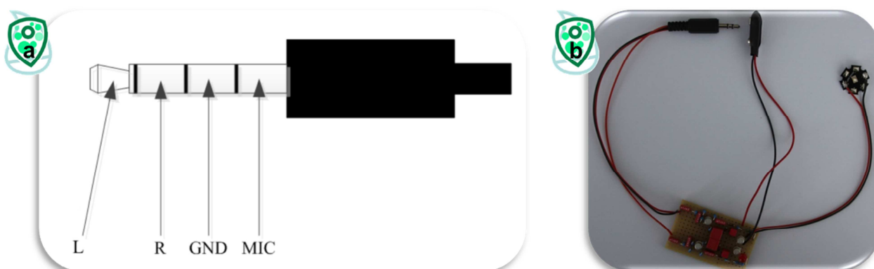
Fig. 11: a) Assignment of earphone plug-in: L = left channel, R = right channel, GND = ground, MIC = microphone and b) Finished circuit board including connections to LED, battery clip and earphone plug-in. Image courtesy a) Produced with MS Visio by Christopher John and b) Anna Friedrichs.
