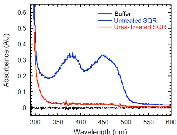
**Supplementary Figure S4.** Absorption spectra of untreated SQR and urea-treated SQR (50  $\mu$ M protomer). The *black trace* is for SQR buffer without reducing reagent: 25 mM Tris-HCl, 500 mM NaCl, 10% glycerol, pH 8.0. The *blue trace* is for untreated SQR and the *red trace* is for urea-treated SQR.
