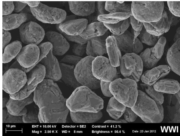
Supplementary Figure 9: SEM image of pristine material. SGN18 graphite under 2,500x magnification.
