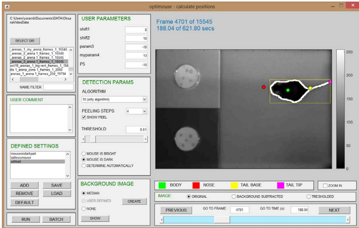
Figure 4.8. Detect GUI with a custom algorithm selected. This algorithm merely imposes a shift on positions detected using one of the built-in algorithms (compare with Figure 4.7). It is intended only for illustration purposes.
