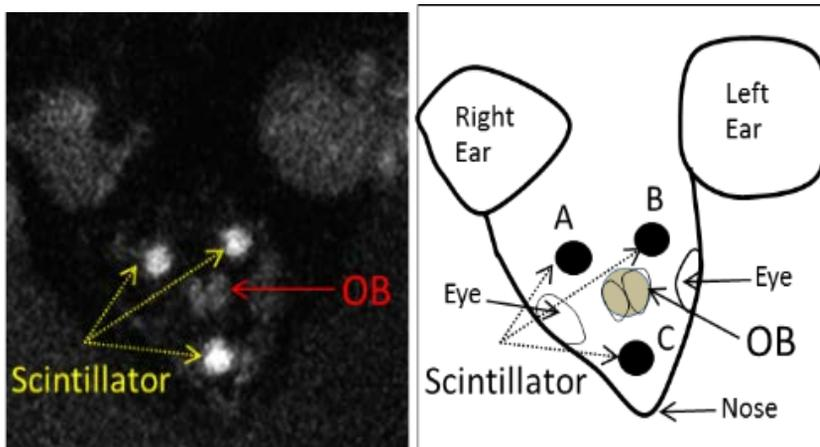
● A,B,C; Scintillator (diameter 2 mm)
