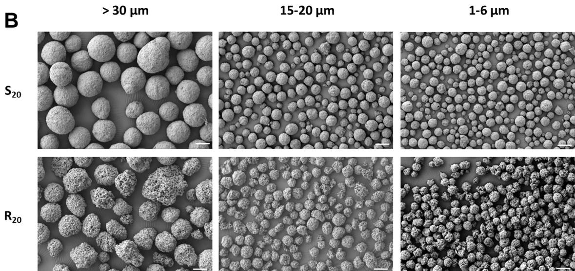
**Supplementary Figure 2.** Hydroxyapatite particles characterization after sieving. Size of HA particles was measured by dynamic light scattering (a); Scanning electron microscopy photomicrographs of  $S_{20}$  and  $R_{20}$  particles after sieving (PluriSelect) (b).
