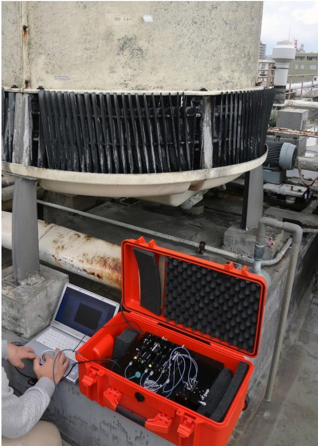
Supplementary Figure S3. On-site monitoring of L. pneumophila in freshwater environment using the portable microfluidic system with a portable battery (i) and in a electric vehicle (ii).
