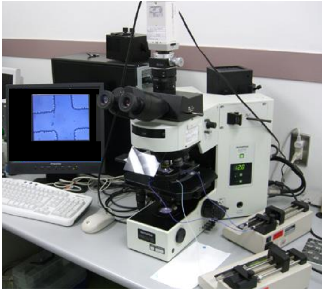
Supplementary Figure S4. Desktop microfluidic system for bacterial monitoring.
