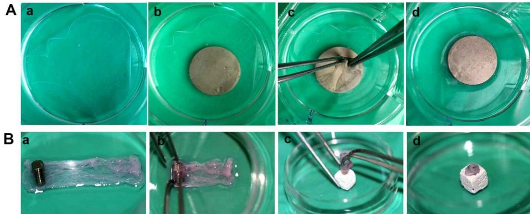
**Supplementary Fig. S3. A: Fabrication of cell sheet-Ti disc complex.** a: Detach cell sheet from plates. b, c: Wrap Ti disc with cell sheet. d: Turn over the complex. **B: Fabrication of cell sheet-implant complex.** a: Fold the cell sheet according to the length of the implant. b: Wrap the implant with cell sheet. c, d: Put the complex into the  $\beta$ -TCP cube.
