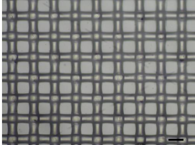
Figure S5. Magnified images of the 100 \mu\text{m} mesh filter (scale bar = 100 \mu\text{m} ). The photograph was captured using a digital SLR camera (Canon EOS Rebel T3) with 50 mm lens (Canon, f/2.5 Compact Macro Lens), cropped and aligned using Microsoft PowerPoint.
