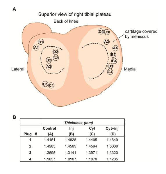
**Supplementary Figure 1. A.** Figure depicting the locations on the tibial plateau where individual explants were taken. **B.** Thickness of the explants used for this manuscript.
