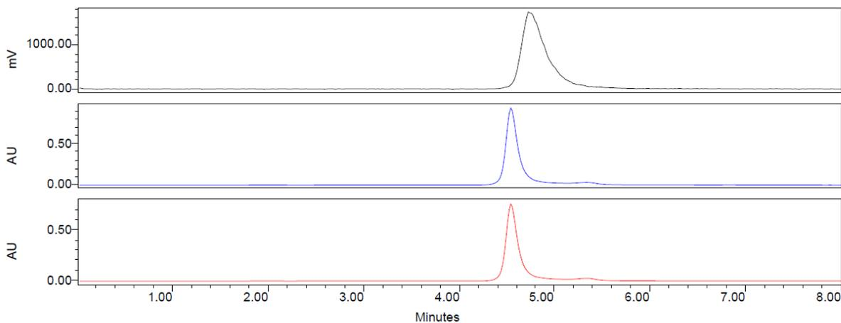
**Co-injection of lorlatinib, (*R*)-1 on analytical HPLC after elution from HLB cartridge and dilution with water (9 mL). Top trace = rad peak and bottom, blue trace = UV @ 254 nm**
