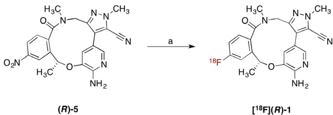
**Supplementary Figure 16.** [<sup>18</sup>F]Fluorination of Nitro precursor **(R)-5** using manual radiosynthesis
