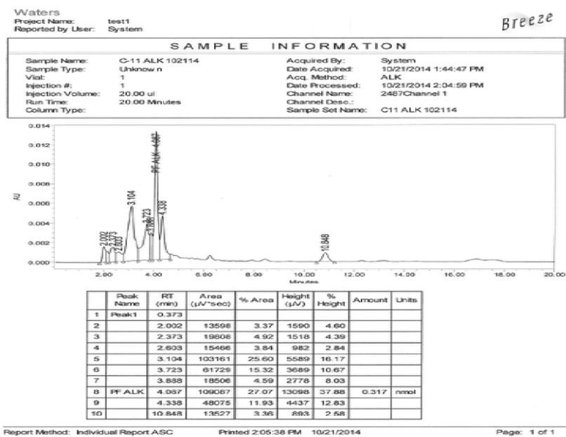
b) Radiation detector HPLC trace of QC sample
