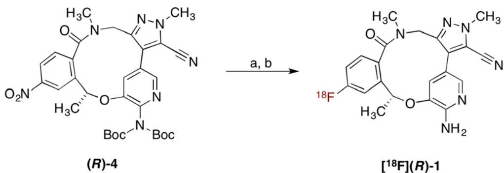
**Supplementary Figure 17.** [<sup>18</sup>F]Fluorination of protected Nitro precursor **(R)-4** using microfluidic radiosynthesis
