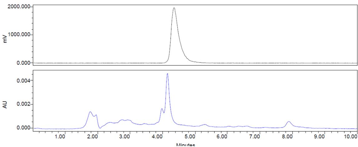
**Analytical HPLC of [<sup>18</sup>F]lorlatinib, (R)-1, after elution from HLB cartridge and dilution with water (9 mL). Top trace = rad peak and bottom, blue trace = UV @ 254 nm**
