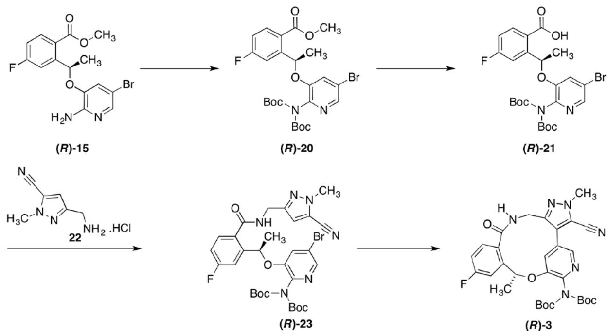
**Supplementary Figure 3.** Synthesis of Protected  $^{11}\text{C}$ -Labelling Precursor, **(R)-3**
