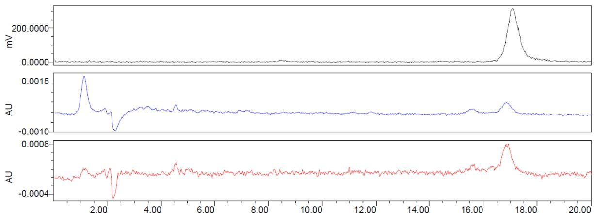
**Analytical HPLC of eluted ethanol solution from C18-Sep-Pak. Top – Rad, Middle = UV @ 254nm and bottom = UV @ 290 nm**
