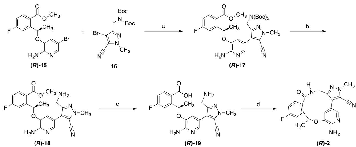
**Supplementary Figure 2.** Synthesis of <sup>11</sup>C-Labelling Precursor, **(R)-2**
