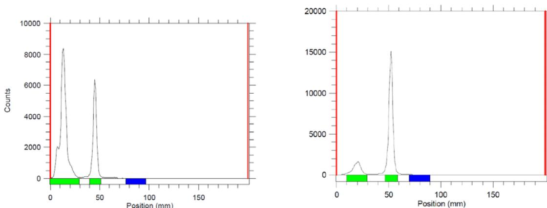
RadioTLC traces of crude reaction mixture (left) and [ $^{18}\text{F}$ ]lorlatinib, (**R**)-**1**, after elution from a C18 SPE. Radiochemical conversions are provided in the table below (% RCC).
