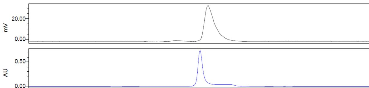
**Coinjection of cold lorlatinib with [<sup>18</sup>F]lorlatinib, (*R*)-1, on analytical HPLC after elution from HLB cartridge and dilution with water (9 mL). Top trace = rad peak and bottom, blue trace = UV @ 254 nm**
