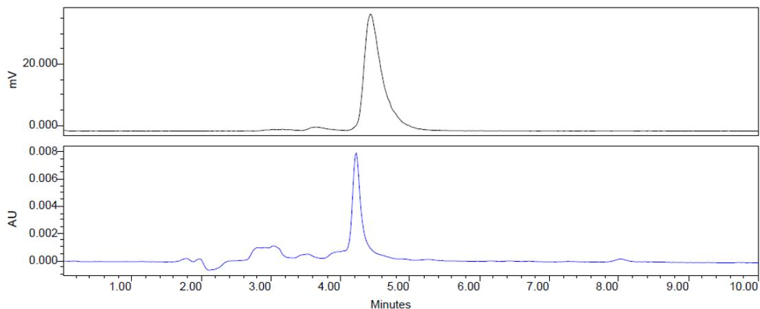
**Analytical HPLC of  $[^{18}\text{F}]$ lorlatinib (*R*)-1 after elution from HLB cartridge and dilution with water (9 mL).** Top trace = rad peak and bottom, blue trace = UV @ 254 nm. 50  $\mu$ L injection. Radio concentration = 310  $\mu$ Ci/ mL @ 1:44 pm
