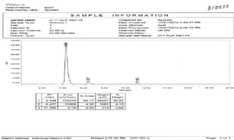
c) UV HPLC trace of QC sample with Standard added to confirm compound
