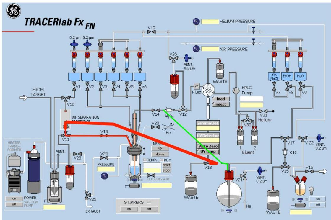
Supplementary Figure 13. Modified flow path of GE TracerLab Fx<sub>FN</sub>
