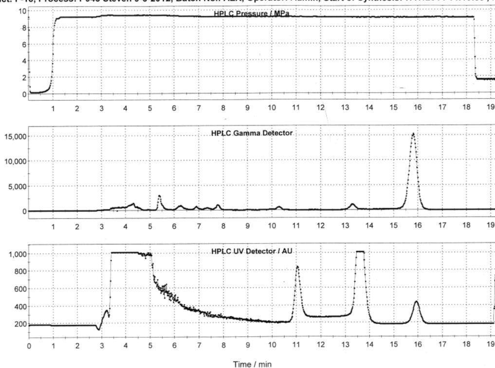
**Supplementary Figure 14.** Semi-prep purification of labeled protected intermediate on GE TracerLab FX<sub>FN</sub>. (HPLC Column: Phenomenex Luna C-18 semiprep, 10 X 250 mm, 10  $\mu$ m; Flow rate: 5 ml/min; Mobile Phase: ACN:0.1M AMF (60:40)).
