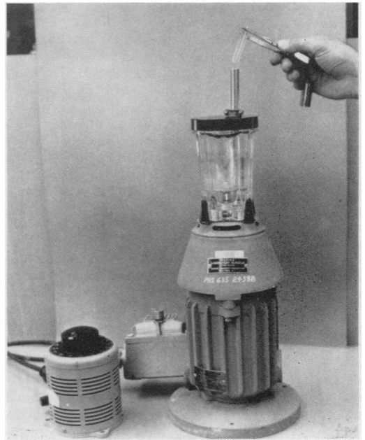
FIG. 3. Modified Waring Blendor jar. The closure for the jar consisted of a threaded lid fitted with a piece of stainless-steel tubing (the entry port) that projected through the lid. A Lucite rod is being aseptically introduced through the entry port to the jar containing 200 ml of sterile acetone.
