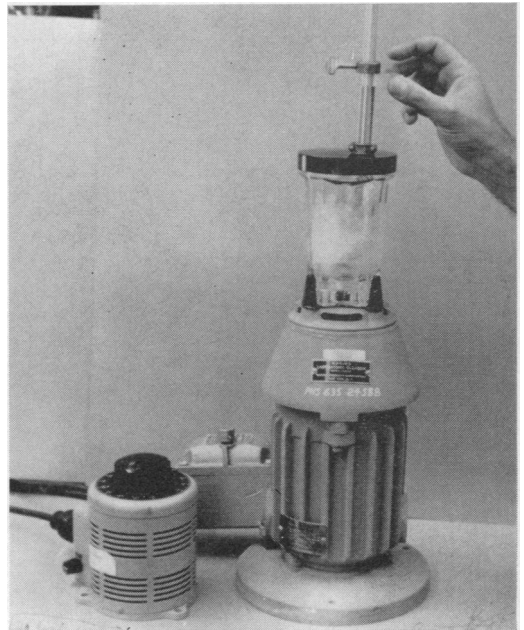
FIG. 5. Plastic rod was dropped down the steel tubing (entry port) of the blender jar, and a sterile steel rod, which acted as a piston to drive the rod against the grinding disc, was inserted.
