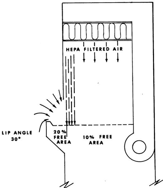
FIG. 4. Schematic cross section of the design mock-up cabinet.
