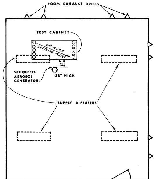
FIG. 1. Setup for product protection tests.
