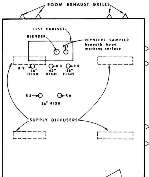
FIG. 2. Setup for agent containment tests.
