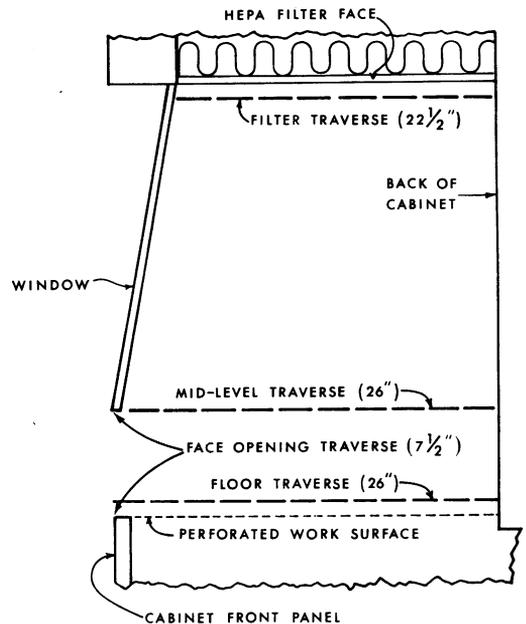
FIG. 3. Measurement locations for velocity profiles.
